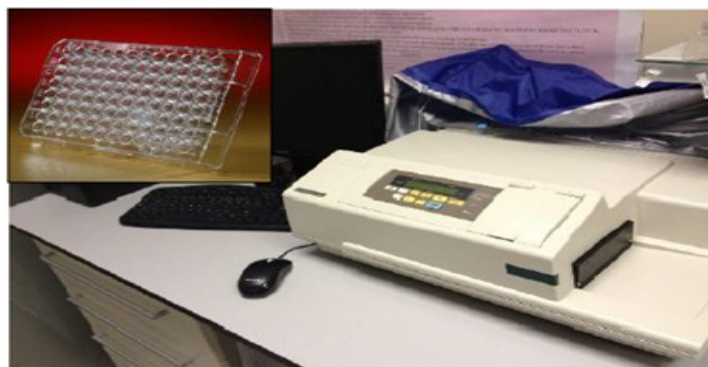
Figure 2.1: Multi mode plate reader (Molecular Devices Spectramax M2) and its 96 well plate
