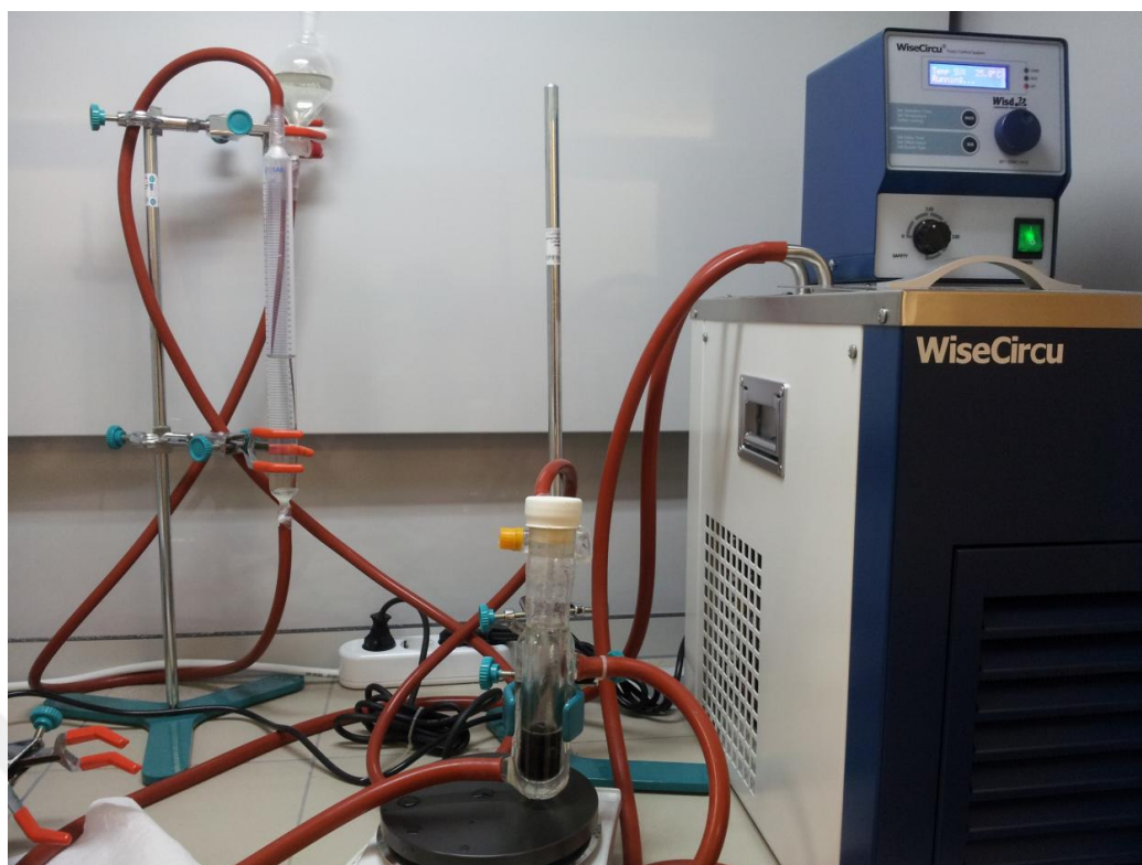
Figure 2.1 System used for the hydrogen production from \text{NH}_3\text{BH}_3 .
