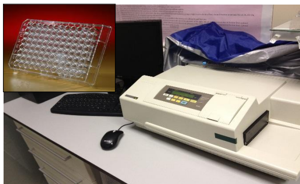
Figure 2.1: Multi mode plate reader (Molecular Devices Spectramax M2) and its 96 well plate.
