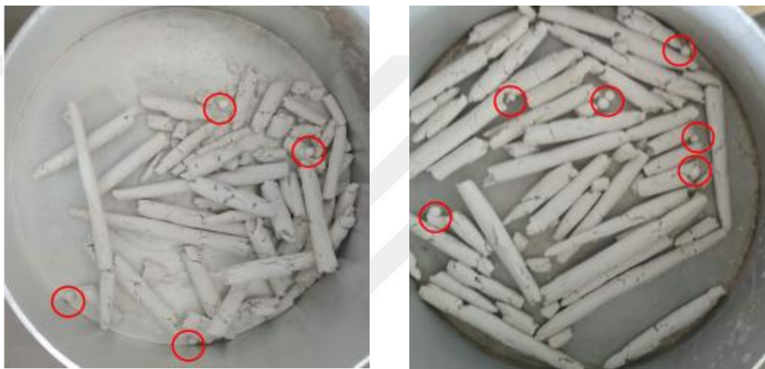
Figure 5.2 Detachment of EPS Beads
