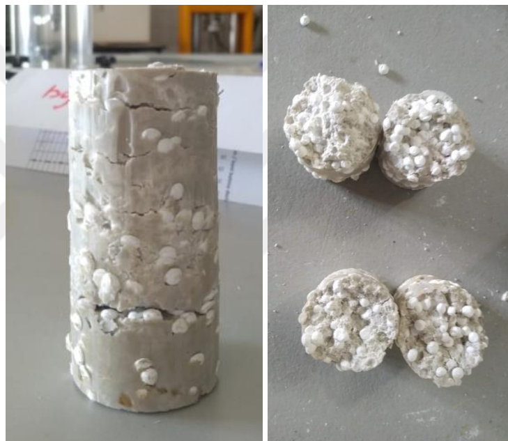
Figure 5.11 Cracks in Sample BG0E2 Due to Segregation
