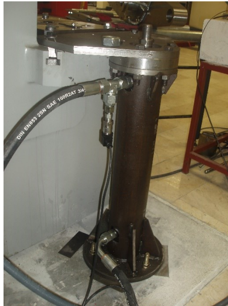
Figure 5.17 Pressure transducer attached on hydraulic cylinder
