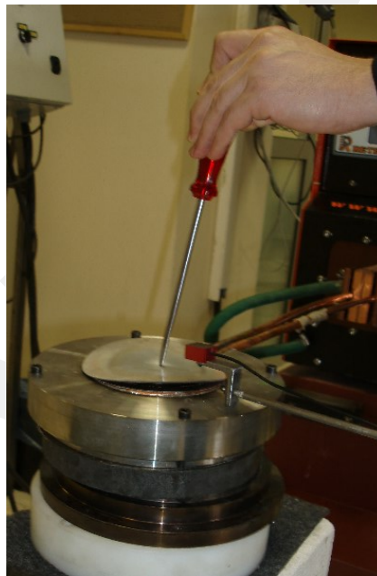
Figure 5.12 Distortion of the blank at warm temperature ( t < 1 mm).
