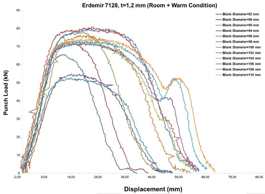
Figure C.22 For Erdemir 7128 (HSLA), t = 1,2 mm, The graph of Punch Load vs Displacement at Room and Warm Conditions.
