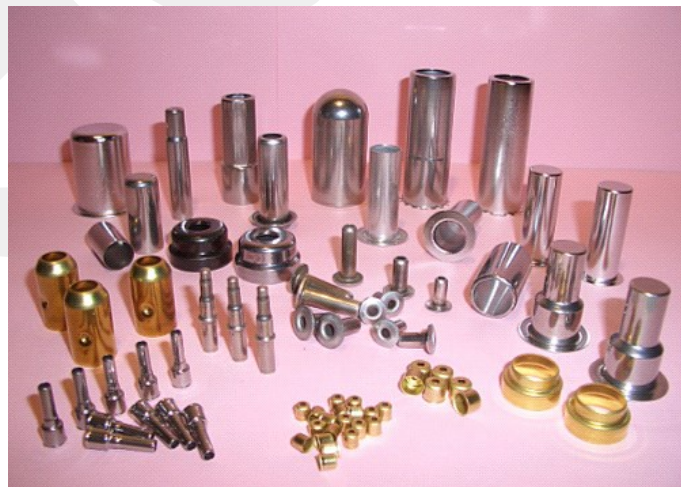
Figure 2.17 Examples to conventional deep drawing workpieces, [43].
