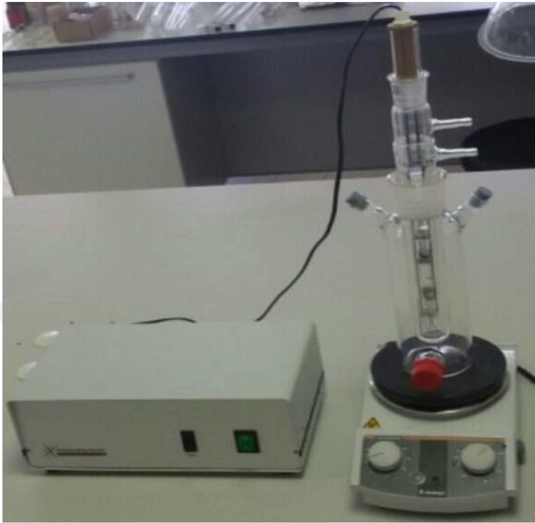
Figure 2.4 UV light exposure system used in this study
