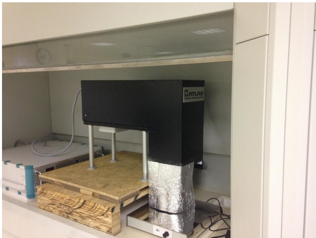
Figure 2.5 Solar simulator used in this study
