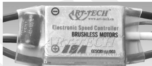
Figure 30 Art-Tech 18A Brushless ESC
