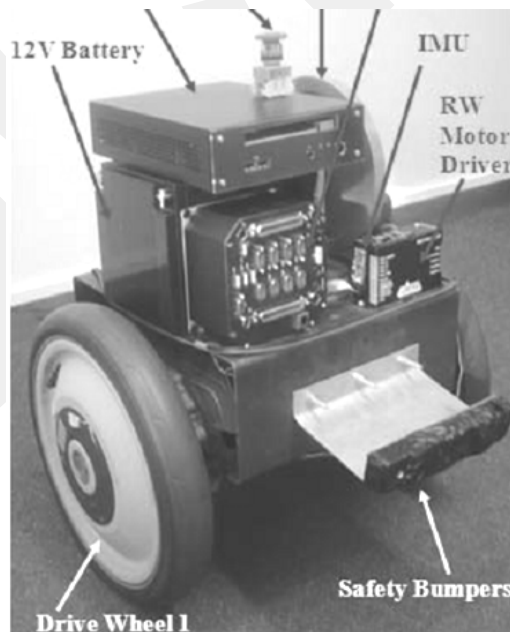
Figure 8 Athena PC 104 System Placed on Two Wheeled Balance System [19]
