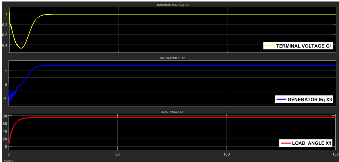
Figure (5-14) load angle ( \delta=75^\circ ), generated voltage Eq and terminal voltage
