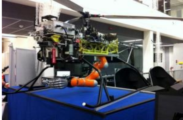
Figure 6: Aerial Robotics Cooperative Assembly System's Preliminary Design [24]
