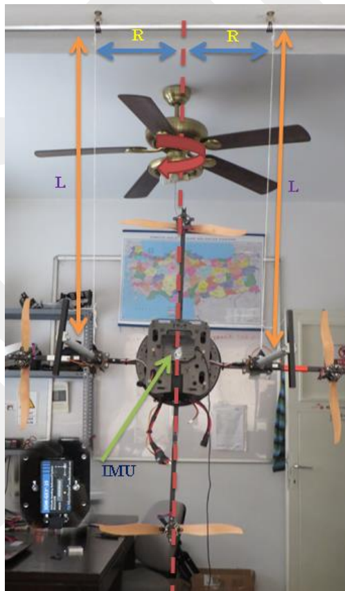
Figure 39: Inertia Test on Roll ( J_{xx} ) axis
