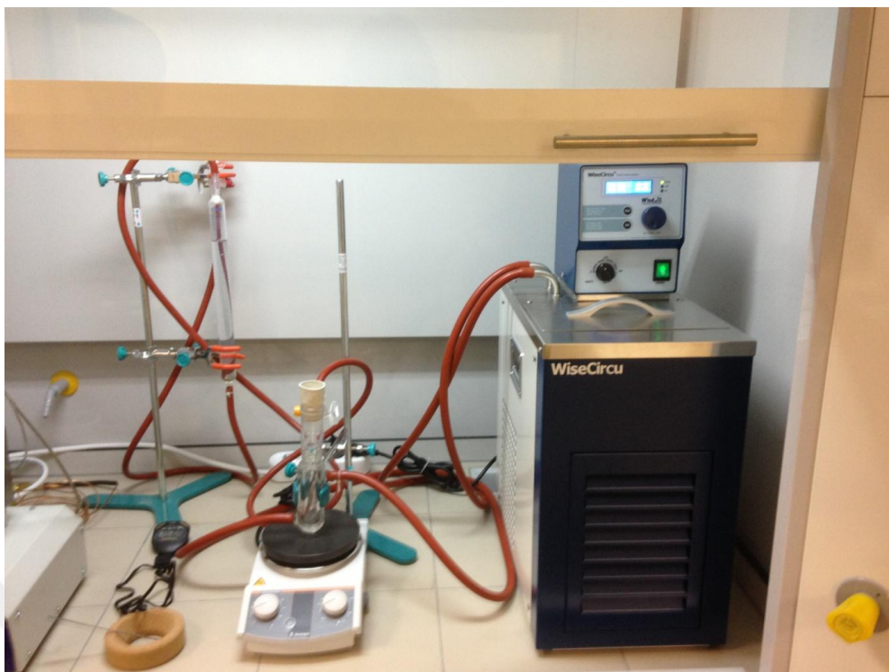
Figure 2.3 System used for the hydrogen production from \text{NH}_3\text{BH}_3 .
