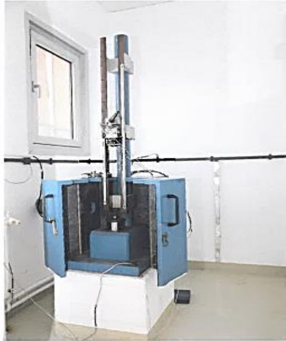
Figure 2.9. BAM Impact Sensitivity Test Device [1]
