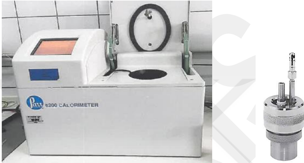
Figure 2.8. Parr 600 calorimeter (left) and Semi-micro oxygen bomb (right) [1]
