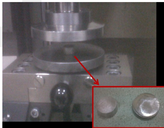
Figure 42: Stack compression test set-up and test specimen
