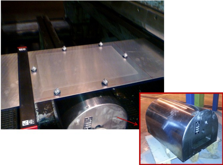
Figure 67: Illustration of the position of sheet metal specimen in stretch forming experiments
