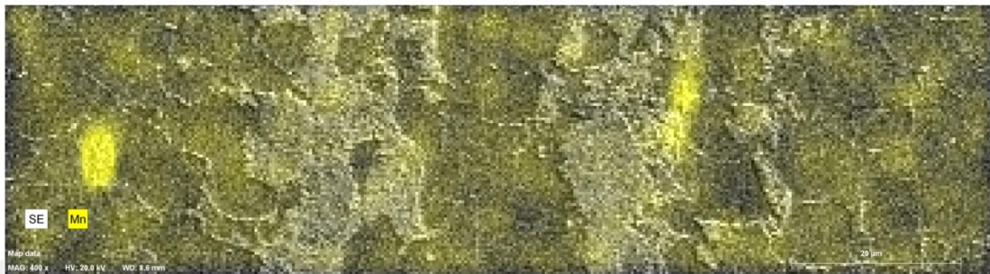
Figure 24. The results of the EDS mapping performed on the area shown in Figure 23 for the 22NiCrMo2-2 steel. The secondary electron micrograph (top) of the region analyzed, and the distribution of Mn (bottom) is given.
