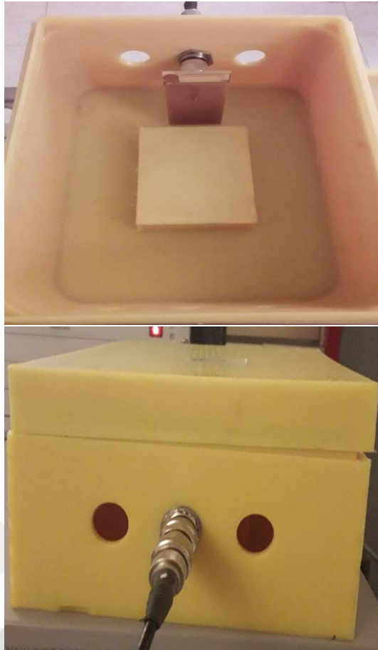
Figure 3.36: Top and side view of the box into which the antenna was placed
