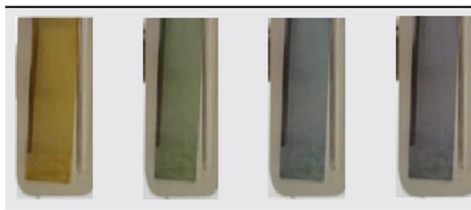
Figure 1.12 The colors of the polymer 12 upon moving from from neutral to oxidized states.
