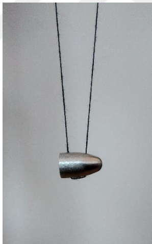
Figure 3.2 Suspended 9 mm bullet model for RCS measurement
