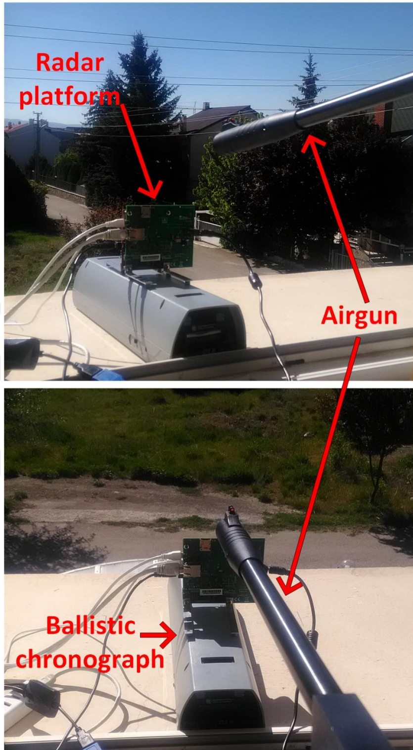
Figure 5.2 Field Experiment Setup with Ballistic Chronograph
