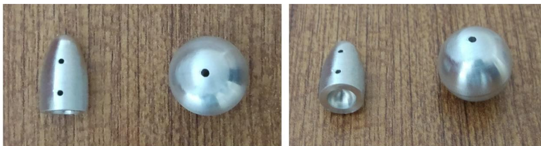
Figure 3.3 Bullet model and 15 mm sphere (holes for suspension threads visible) Top view and 45° angle view (from rear side)
