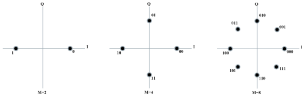
Figure 2.6 PSK Constellation Diagram [81]
