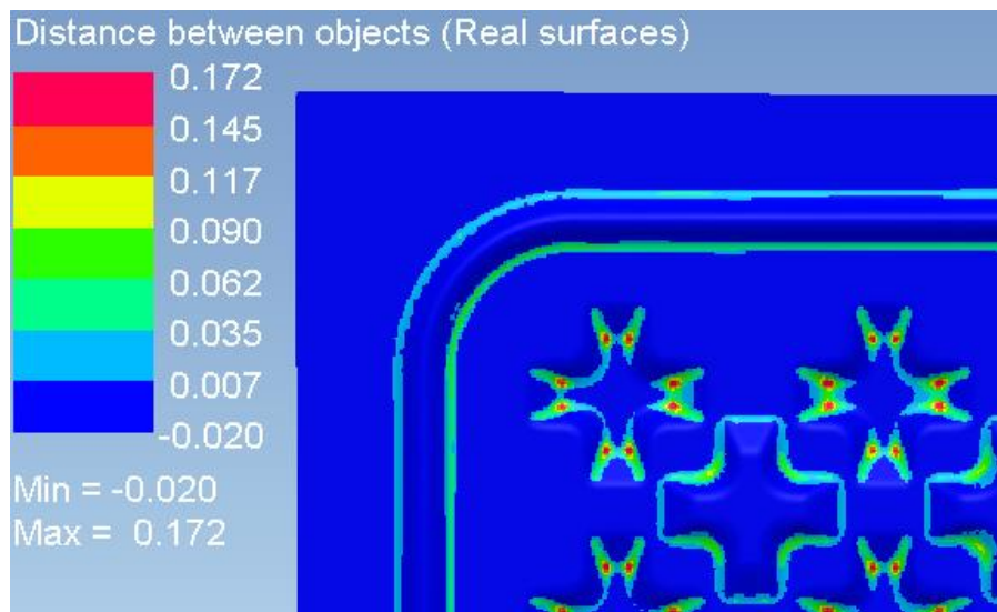
Figure 4.36 The distance in between design 22 and die
