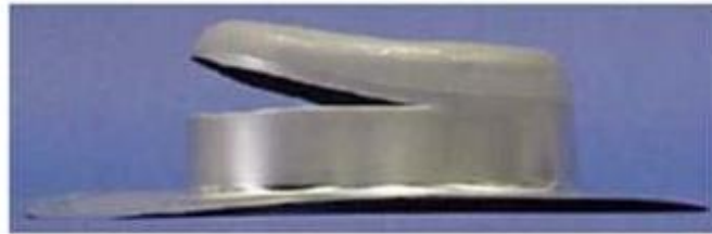
Figure 2.25 An exmple of tearing [2]
