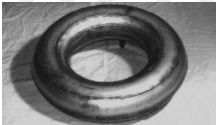
Figure 2.17 Example of Shell Hydroforming [21]
