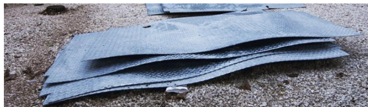
Figure 2.24 An example of warping [26]
