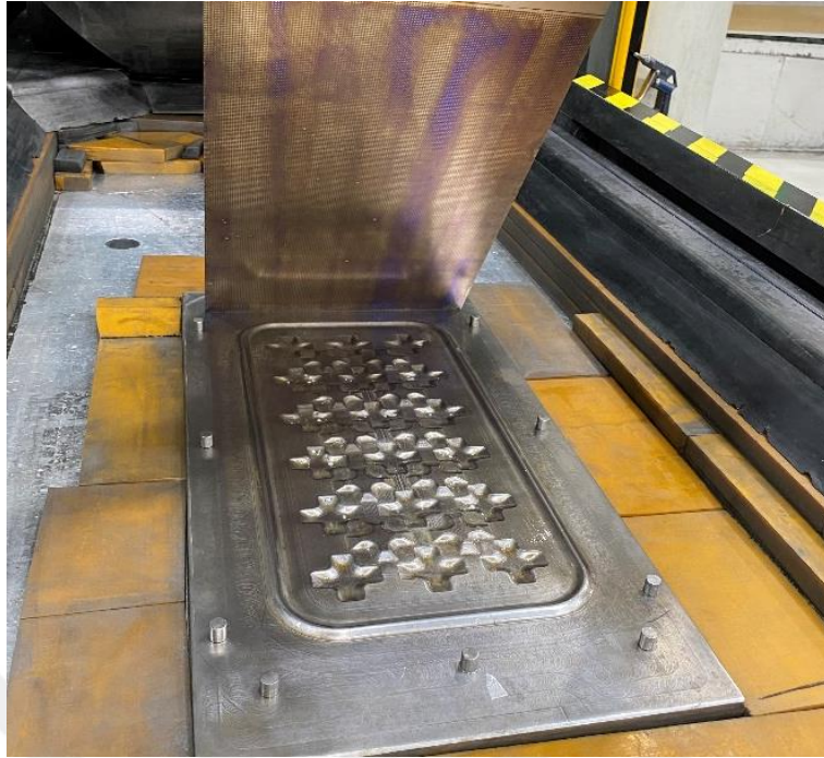
Figure 4.72 Placing the marked face into the mold
