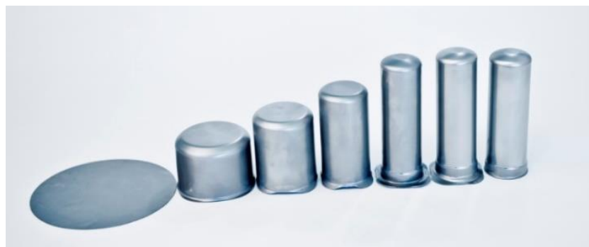
Figure 2.20 Deep Drawing steps [24]
