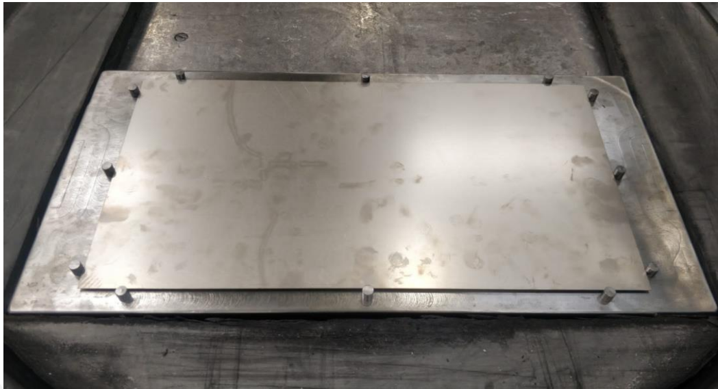
Figure 4.56 placing the part in the mold
