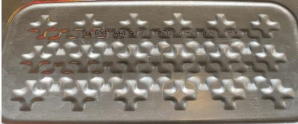
Figure 4.58 Deformed sheet-shaping patterns
