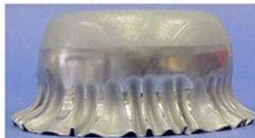
Figure 2.21 An example of wrinkling [2]
