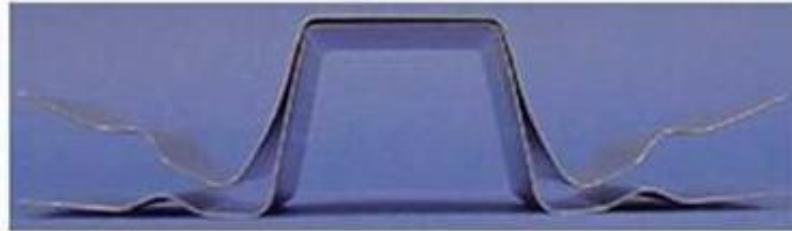
Figure 2.22 An example of springback [2]
