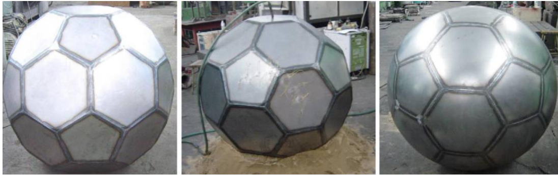
Figure 2.18 Example of Shell Hydroforming [22]
