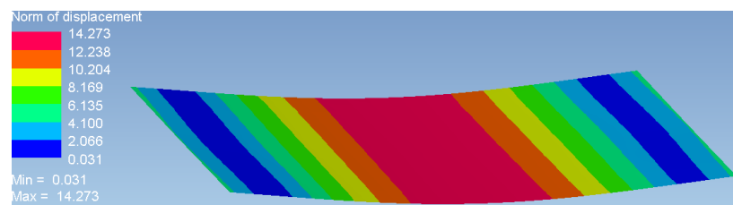
Figure 4.38 The unformed part deflection under 5N
