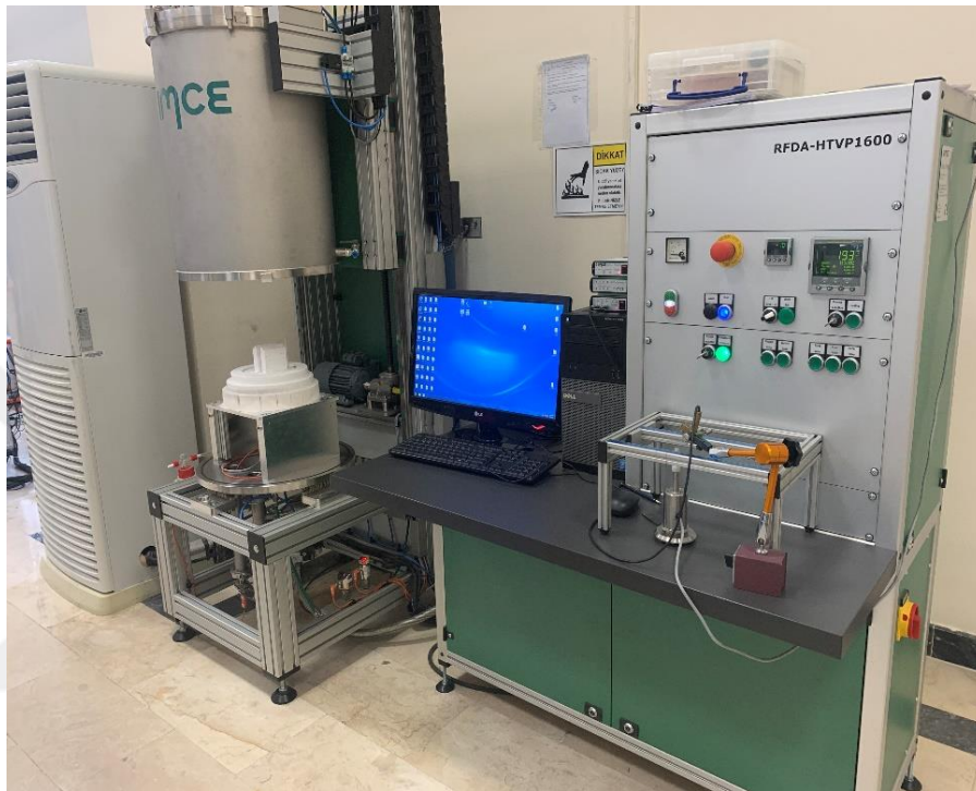
Figure 3.3 IMCE RFDA-HTVP 1600 Device
