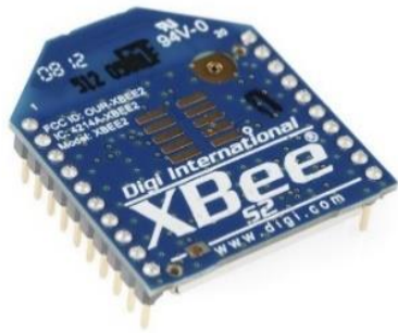
Figure 18: Xbee Series 2 and USB Dongle
