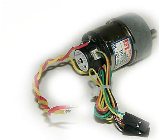
Figure 21: HN-GH12-1634T-30:1 DC motor
