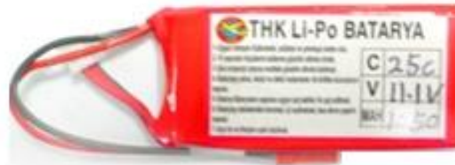
Figure 23: THK 11.1 V Li-Po Battery
