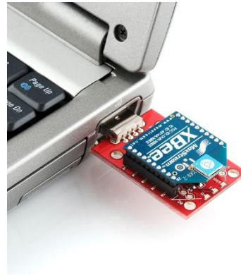
Figure 18: Xbee Series 2 and USB Dongle
