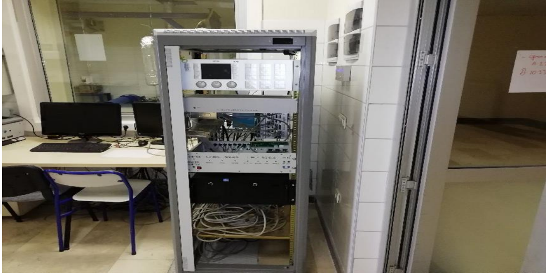
Figure 3.2: Single cylinder test control console.
