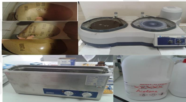
Figure 2. 5 Grinding, polishing, cleaning, and etching processes
