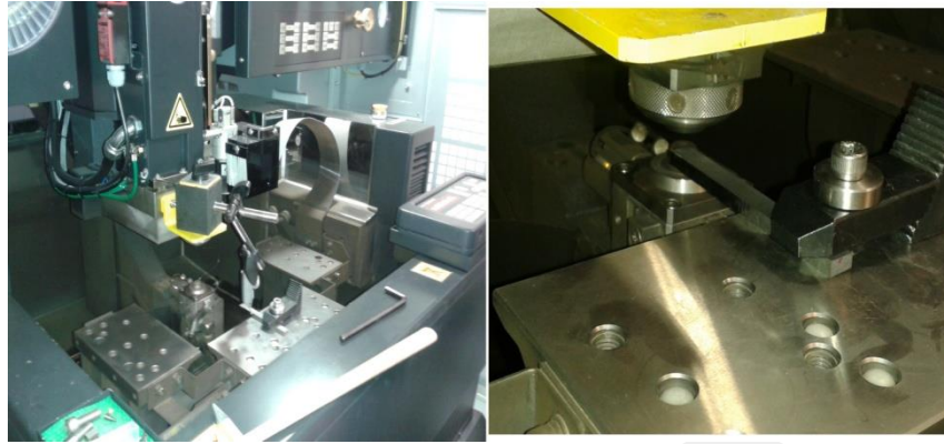
Figure 2. 2 \mu -WEDM (Sodick AP250L) used to conduct the experiments on the Nitinol alloy sample
