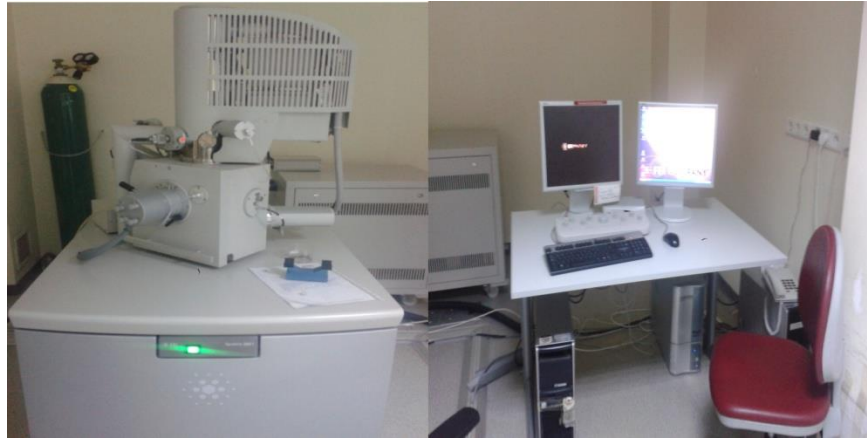
Figure 2. 13 SEM quanta 200f with EDS unit used to scan the white recast layer
