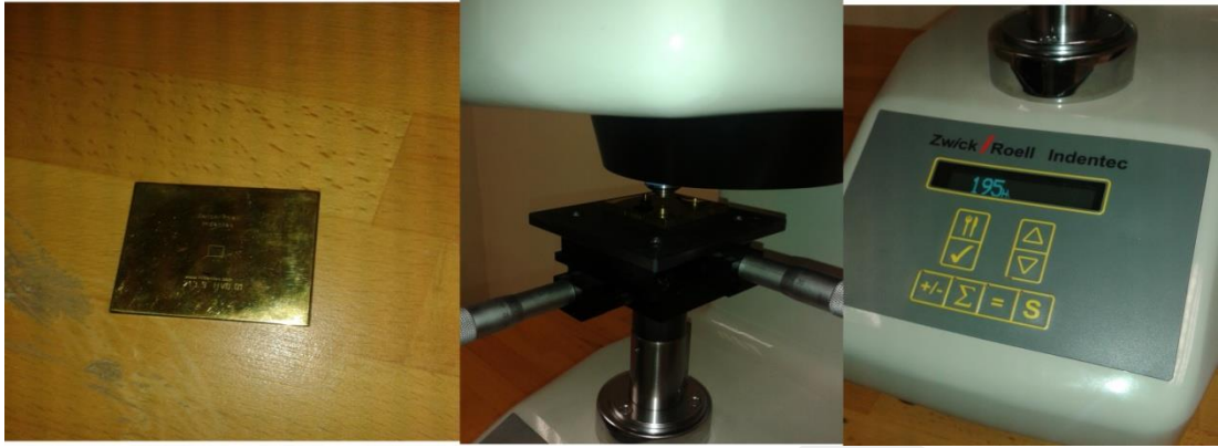
Figure 2. 33 Micro-hardness ZWICK.ROELL ZHv \mu calibration
