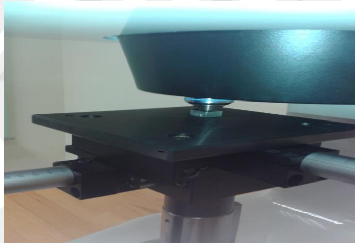
Figure 2. 34 Measuring of bulk material micro-hardness
