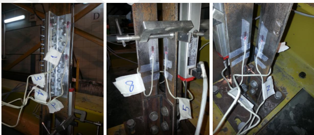
Figure 2.40. Members instrumented with strain gages (Specimen-2)
