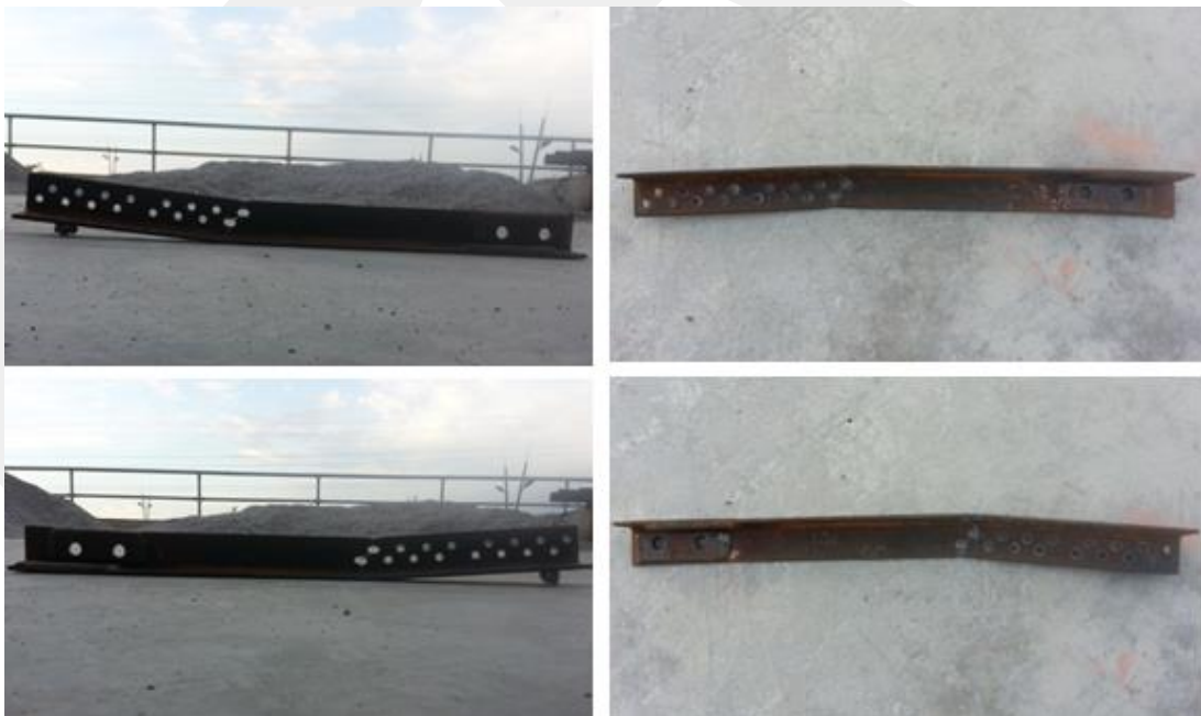
Figure 2.50. Bending of ruptured angle member of Specimen-3
