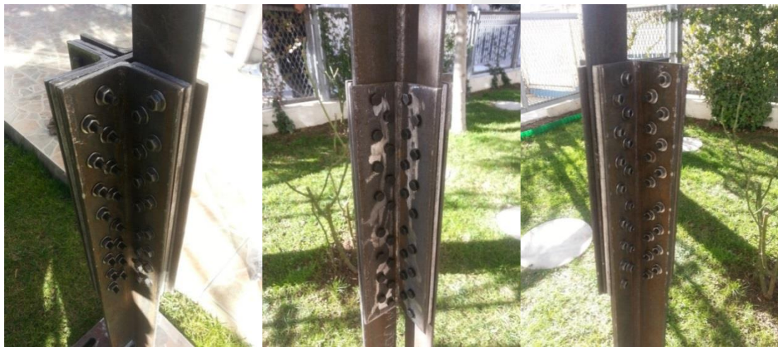
Figure 2.13. Members and connection detail of Specimen-1
