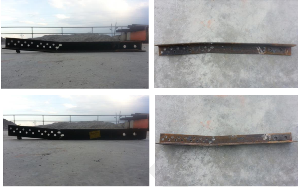
Figure 2.97. Bending of ruptured main member of Specimen-7
