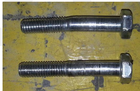
Figure 2.82. Bending deformation on bolts (Specimen-6)
