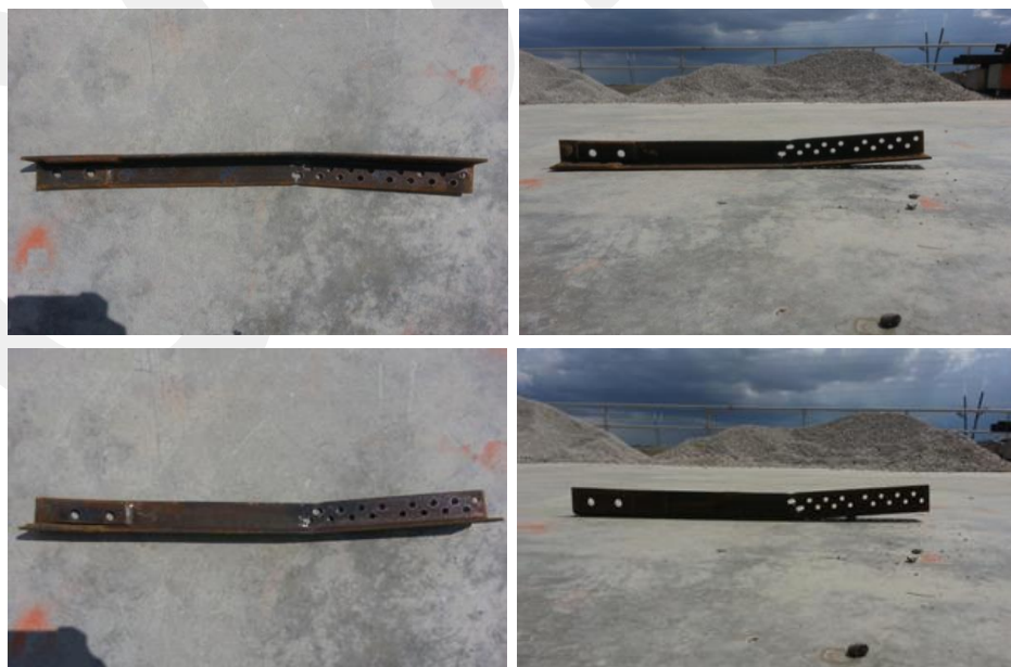
Figure 2.59. Bending of ruptured angle member of Specimen-4
