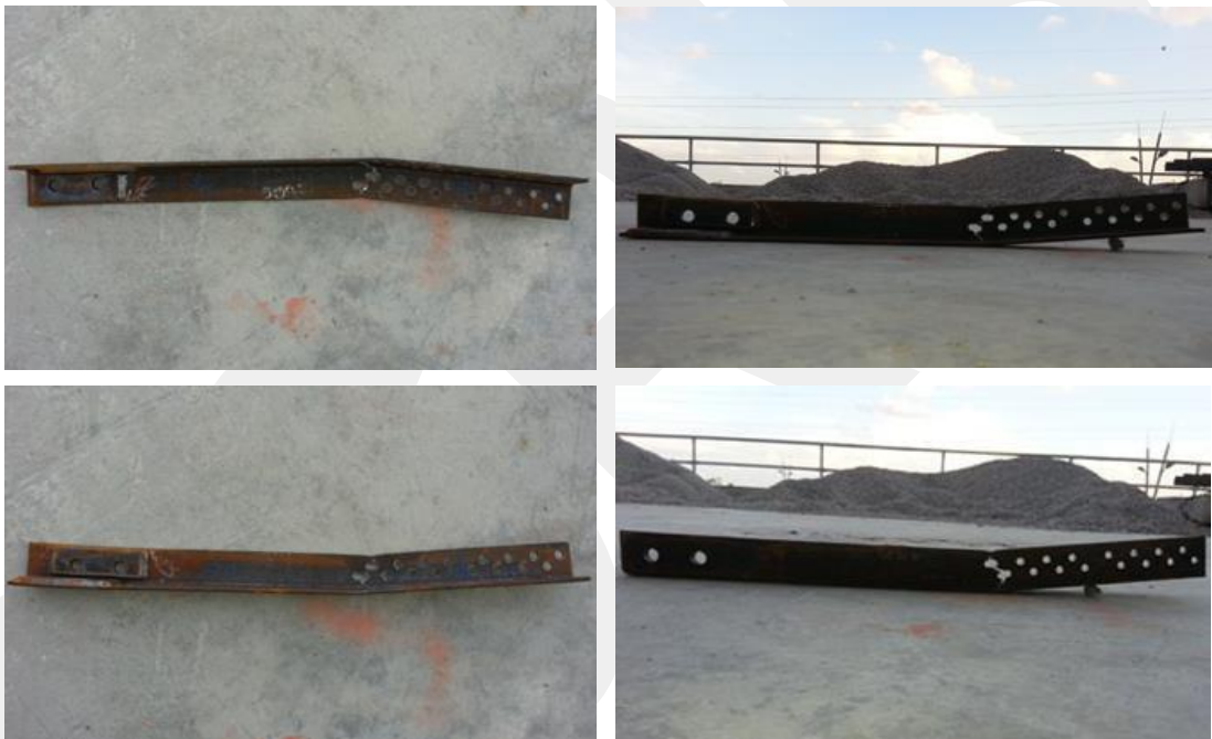
Figure 2.73. Bending of ruptured angle member of Specimen-5
