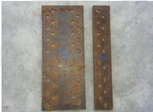
Figure 2.86. Filler plates of Specimen-6, after testing
