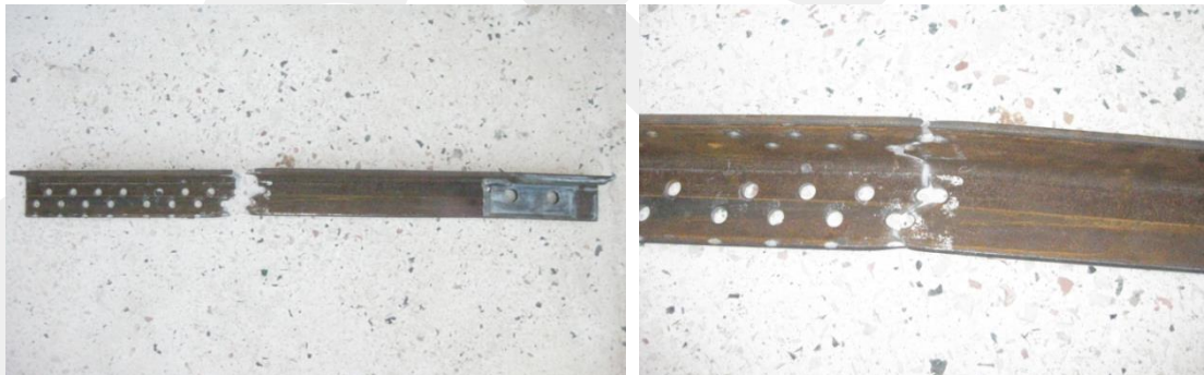
Figure 2.31. Deformations on ruptured angle member of Specimen-2
