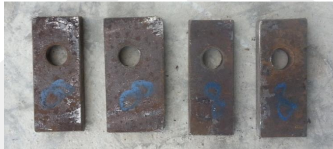
Figure 2.98. Filler plates of Specimen-7, after testing
