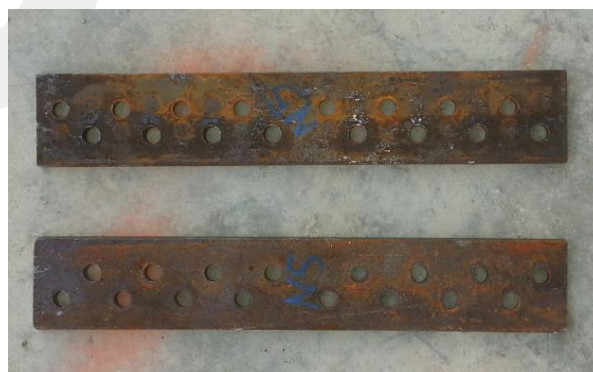
Figure 2.74. Filler plates of Specimen-5, after testing
