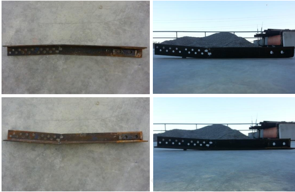
Figure 2.85. Bending of ruptured main member of Specimen-6
