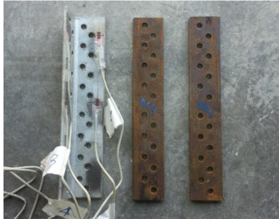
Figure 2.60. Reinforcement angle members and filler plates of Specimen-4, after testing
