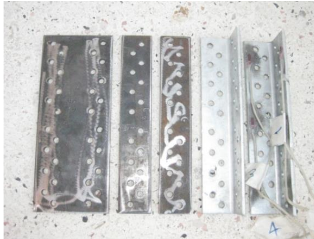
Figure 2.32. Reinforcement angle members and filler plates of Specimen-2, after testing
