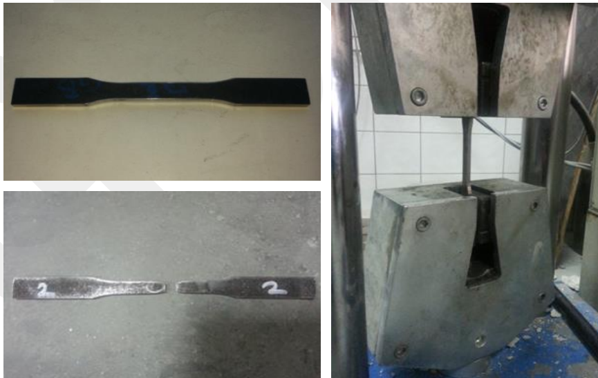
Figure 2.9. Tension test coupons and testing procedure
