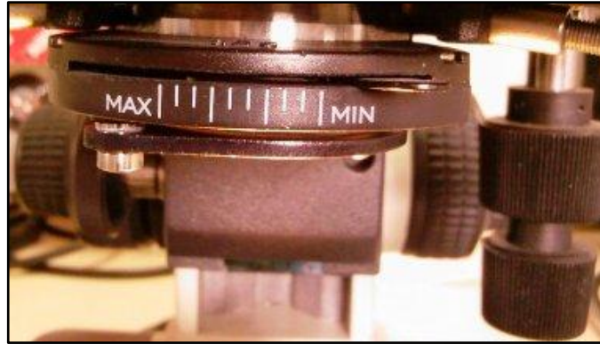
Figure 31. Slider control unit for the light power of microscope.
