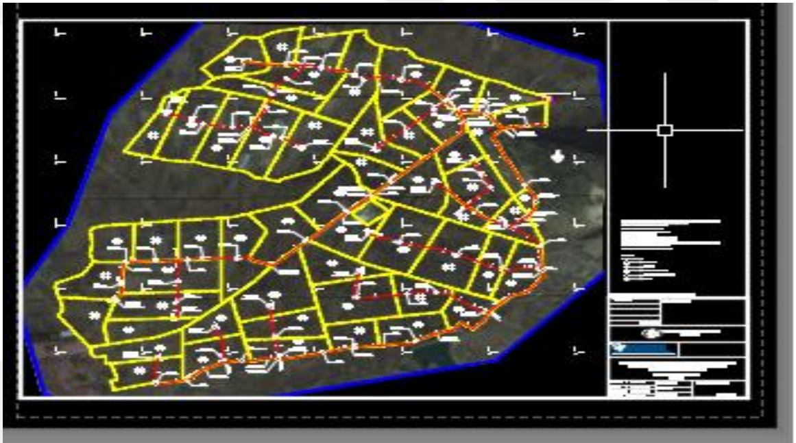
Figure 5-1 Area plan view of the Atabey project layout drawn by AutoCAD
