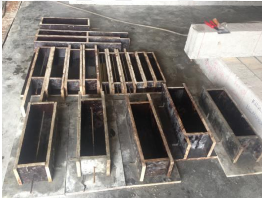
Figure 3-6 – Formworks for 60×60×500, 100×100×500, and 150×150×500 mm beam specimens before casting
