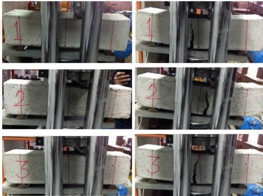
Figure 4-3 – Typical failure mode of CC prisms under flexure 1
