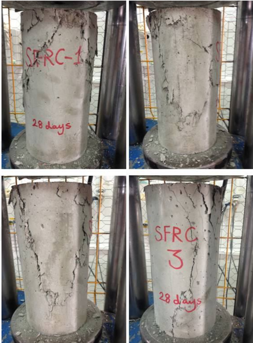
Figure 4-2 – Typical failure mode of SFRC cylinders under compression
