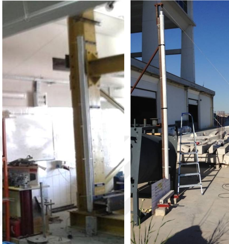
Figure 3-23 – Drop-hammer testing apparatus at different locations (indoors and outdoors)
