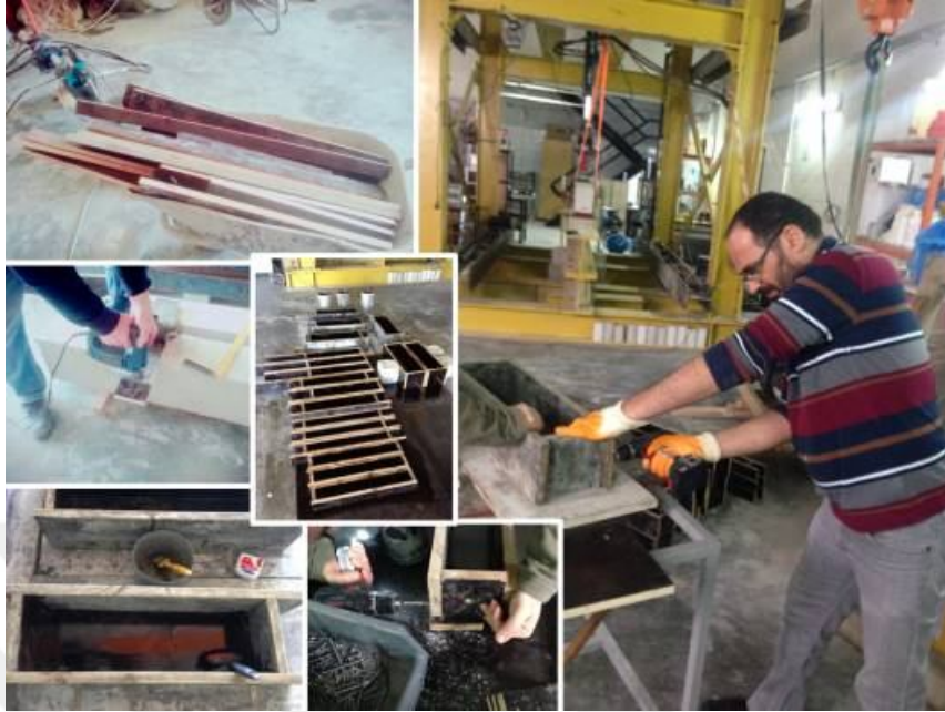
Figure 3-5 – Preparations of formworks for 60×60×500, 100×100×500, and 150×150×500 mm beam specimens
