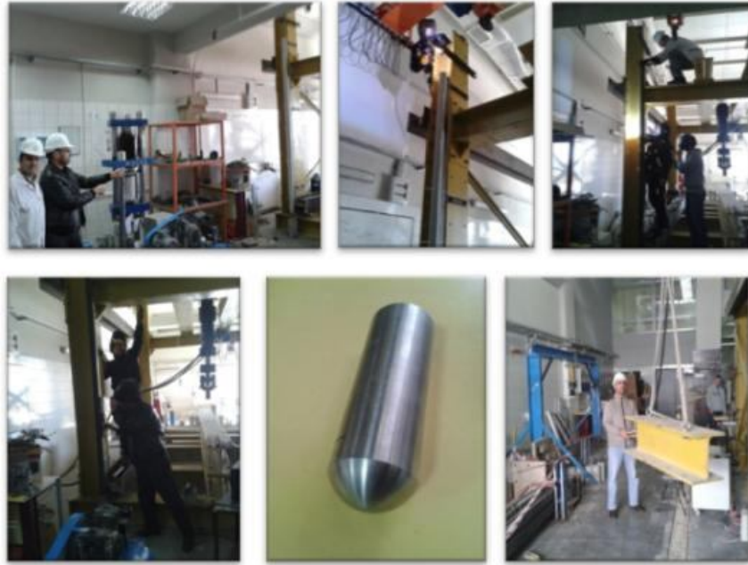
Figure 3-20 – Construction process of the drop-hammer testing apparatus
