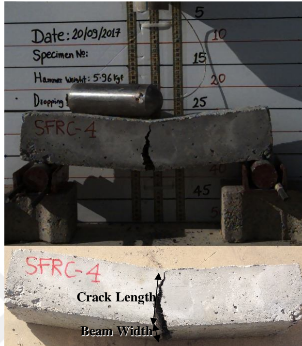
Figure 5-67 – Definitions for crack length and beam width
