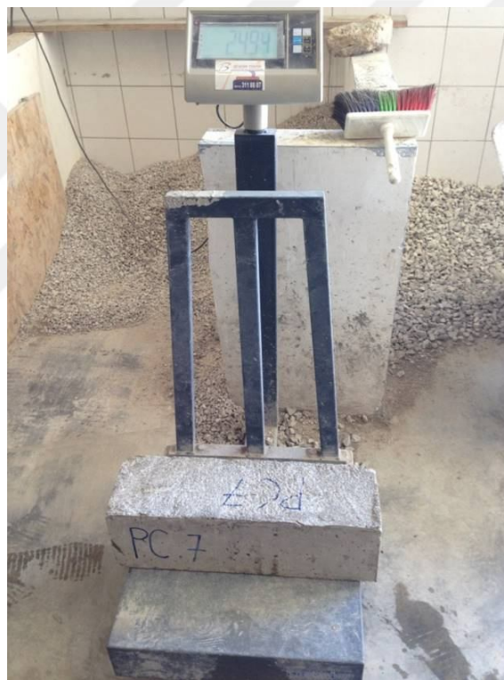
Figure 5-9 – Measurement of specimens weight at laboratory to determine its density
