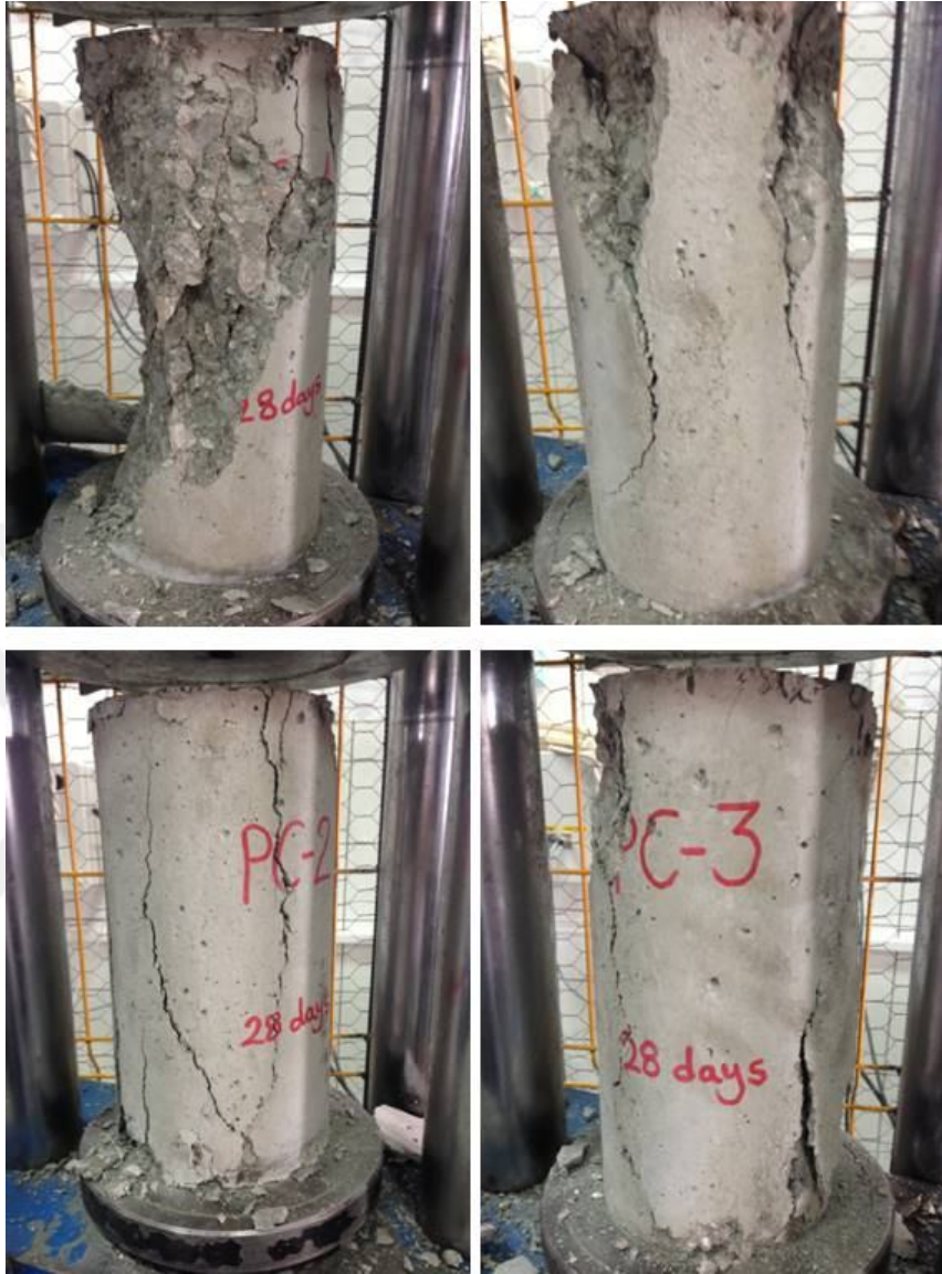
Figure 4-1 – Typical failure mode of CC cylinders under compression
