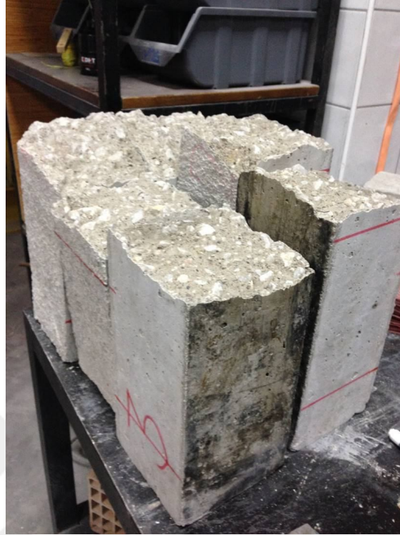
Figure 4-4 – Typical failure mode of CC prisms under flexure 2
