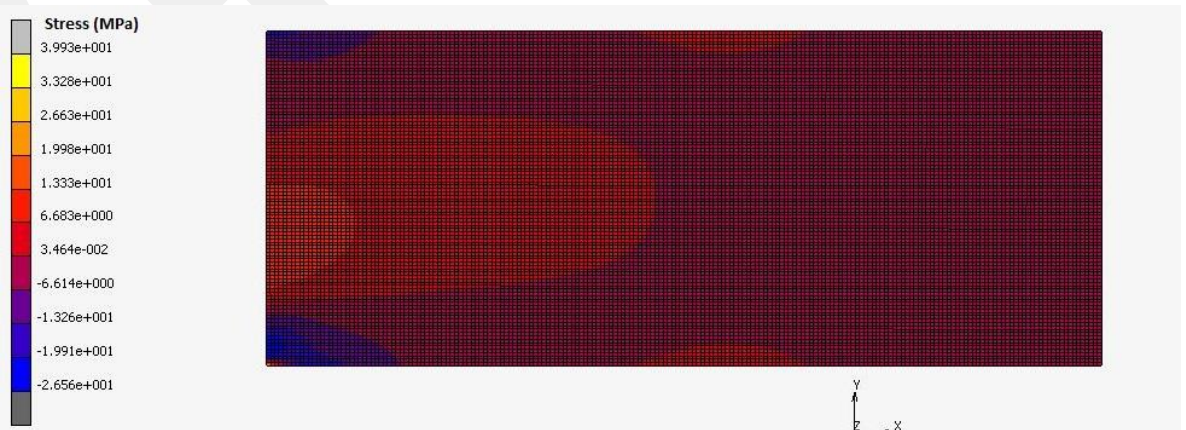
Figure 28: Stress Distribution on Specimen B5 (2D)
