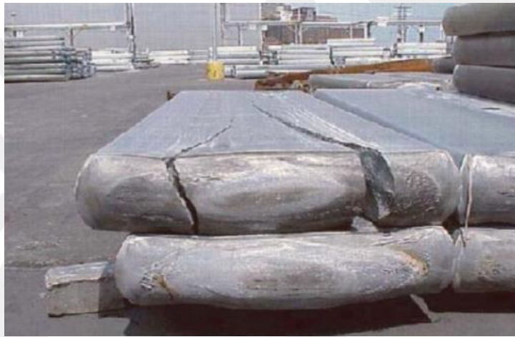
Figure 2: Cracks on a cast aluminum ingot due to excessive residual stresses [6]
