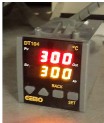
Figure 22. Temperature control device
