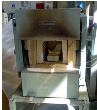
Figure 27. Heat treatment furnace
