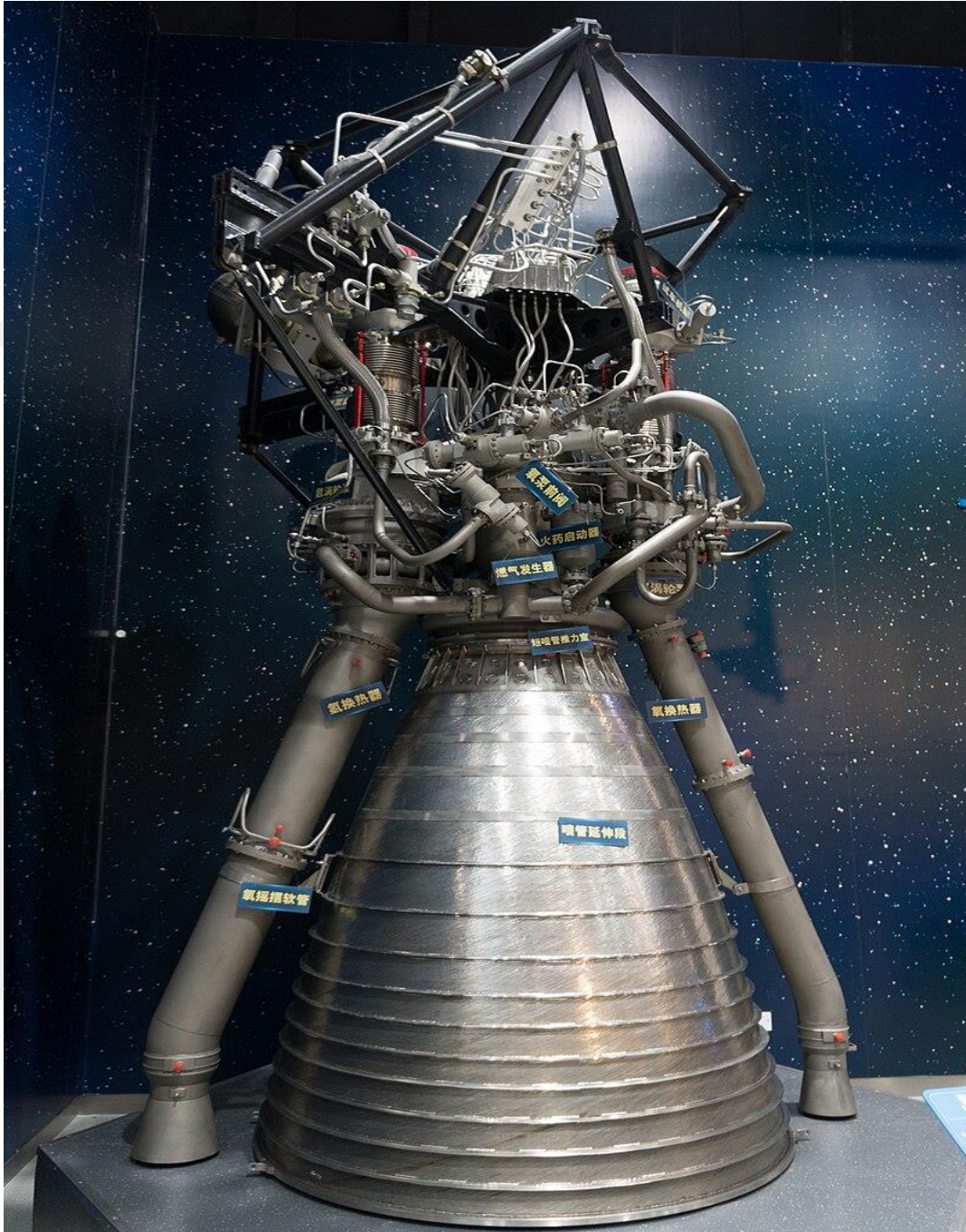
Figure 1.3 Chinese YF-77 Engine Used by Long March 5 [11].
