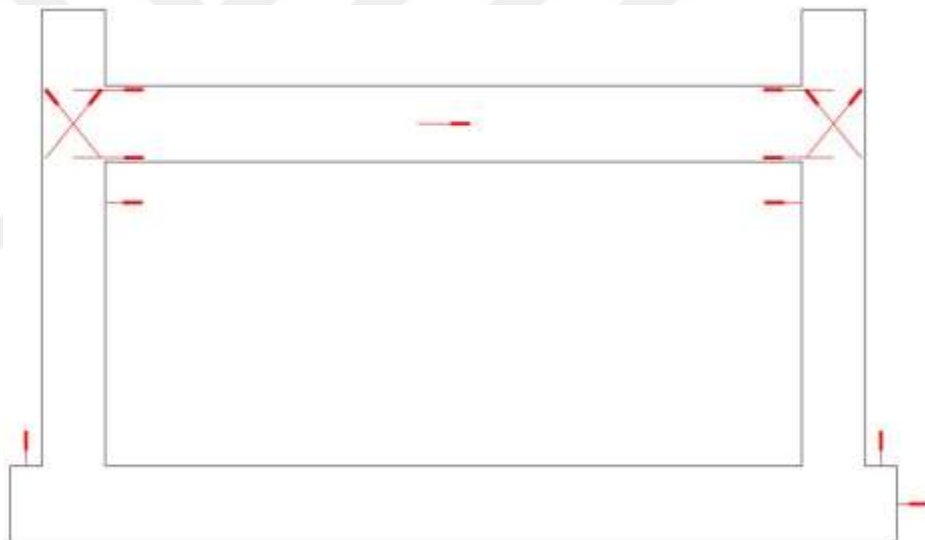
Figure 3.20 The LVDT instrumentation scheme
