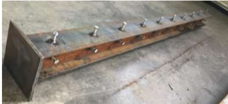
Figure 3.10 HEB100 structural steel section with shear studs
