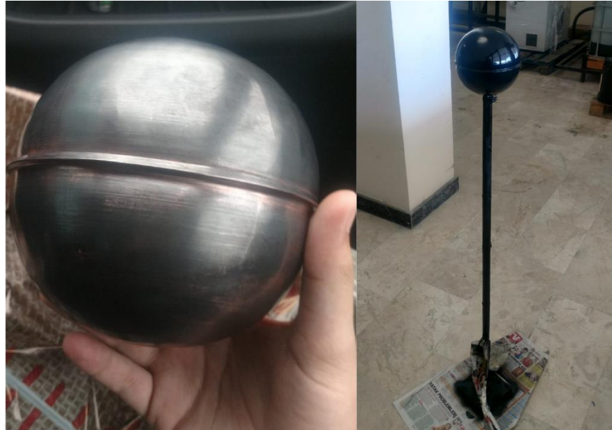
Figure 5.12. Globe Sphere after Construction (on the left) and The Developed Globe Thermometer After Dyeing (on the right).
