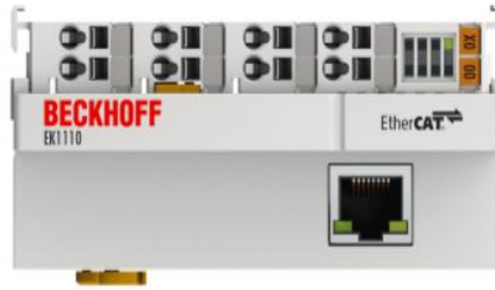
Figure 3.29 EtherCAT Mounted on the Embedded Computer
