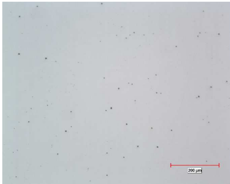
Figure B-13 Inclusion rating of B-Slab13
