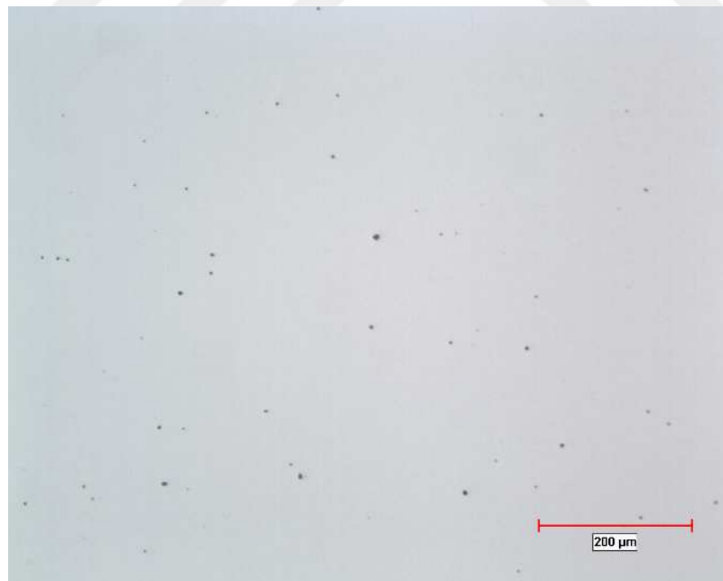
Figure B-5 Inclusion rating of B-Slab3
