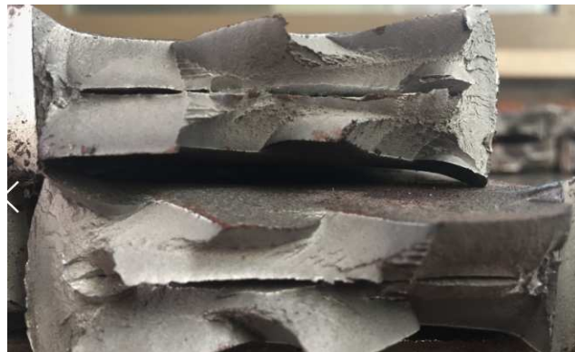
Figure 57 DWTT Result for B-Slab11
