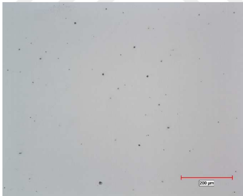
Figure B-3 Inclusion rating of B-Slab2
