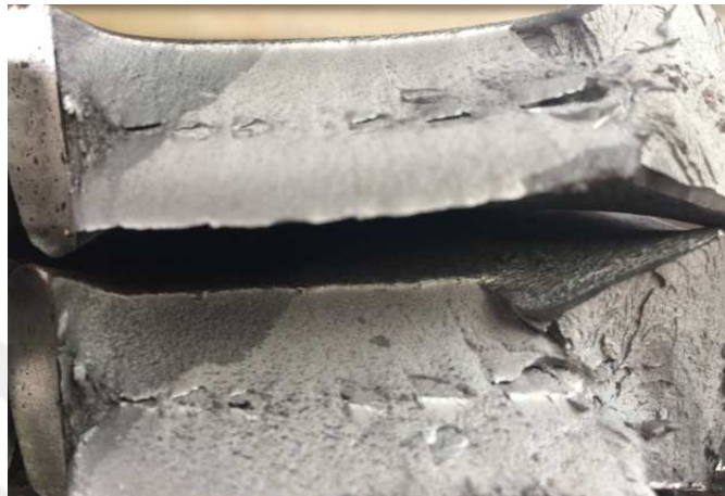
Figure 54 DWTT Result for B-Slab9
