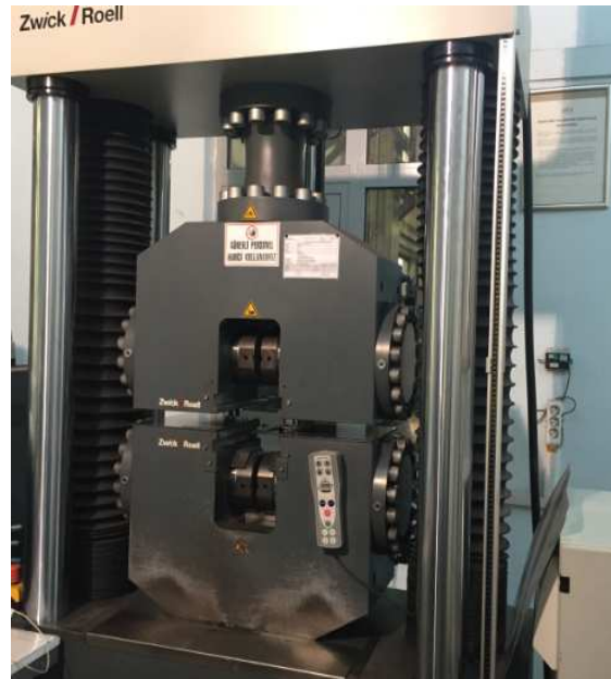
Figure 38 Zwick tensile test machine
