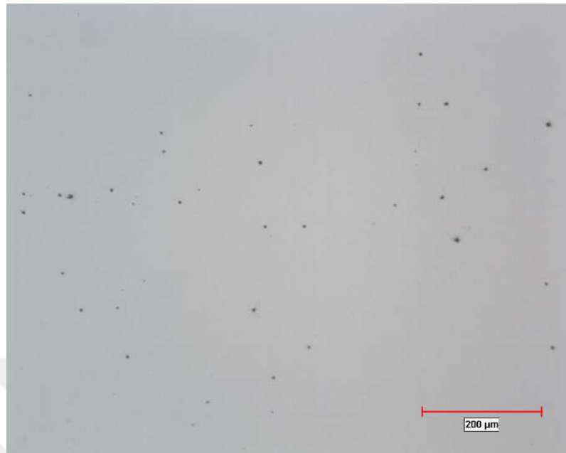
Figure B-8 Inclusion rating of B-Slab5
