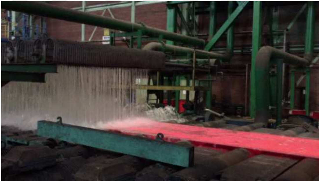
Figure 18 Accelerated cooling of plates using water shower
