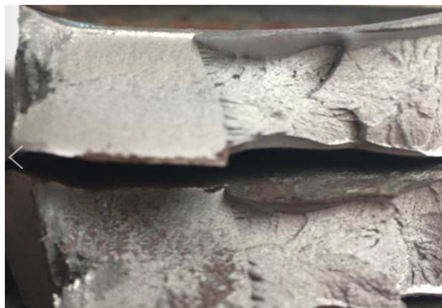
Figure 59 DWTT Result for B-Slab13
