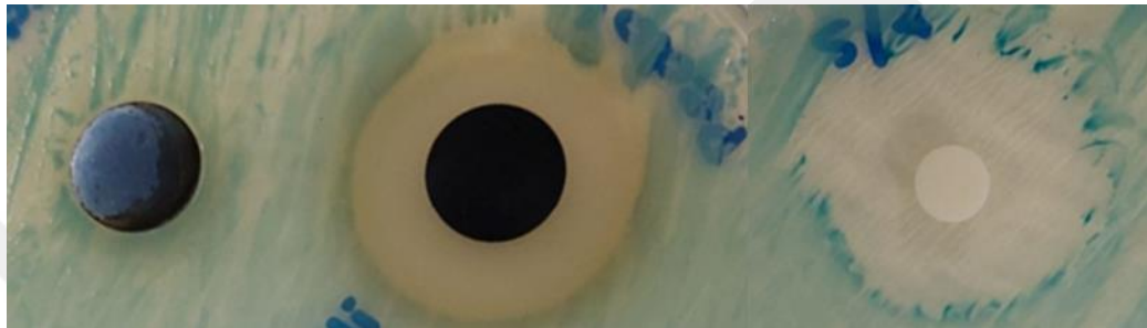
Figure 3.7: (a) PEDOT (b) PEDOT-Ag (c) Pen/strep ( E.coli )
