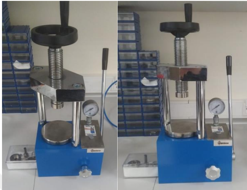
Figure 2.3: A press is used to prepare nanoparticle pellets.
