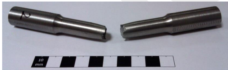
Figure 3.3 Tensile Test Circular Specimen (End of the test)
