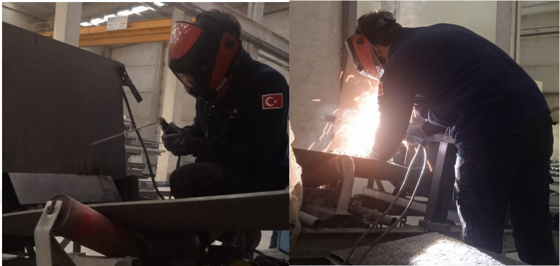
Figure 4.19: Manufacturing of the Chute on the conveyor belt.
