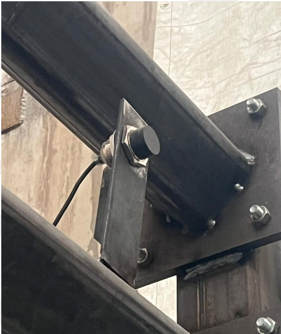
Figure 4.6: Proximity sensor inside the prototype sampling system.
