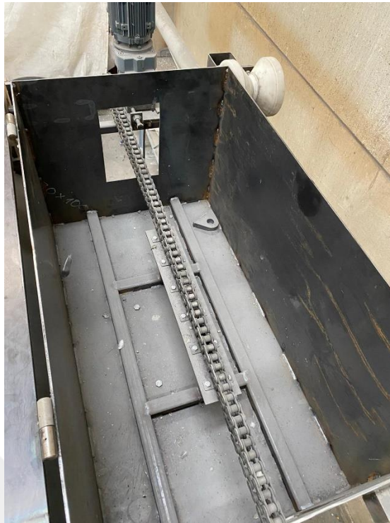
Figure 4.16: Assembling process of gearmotor and chain system.
