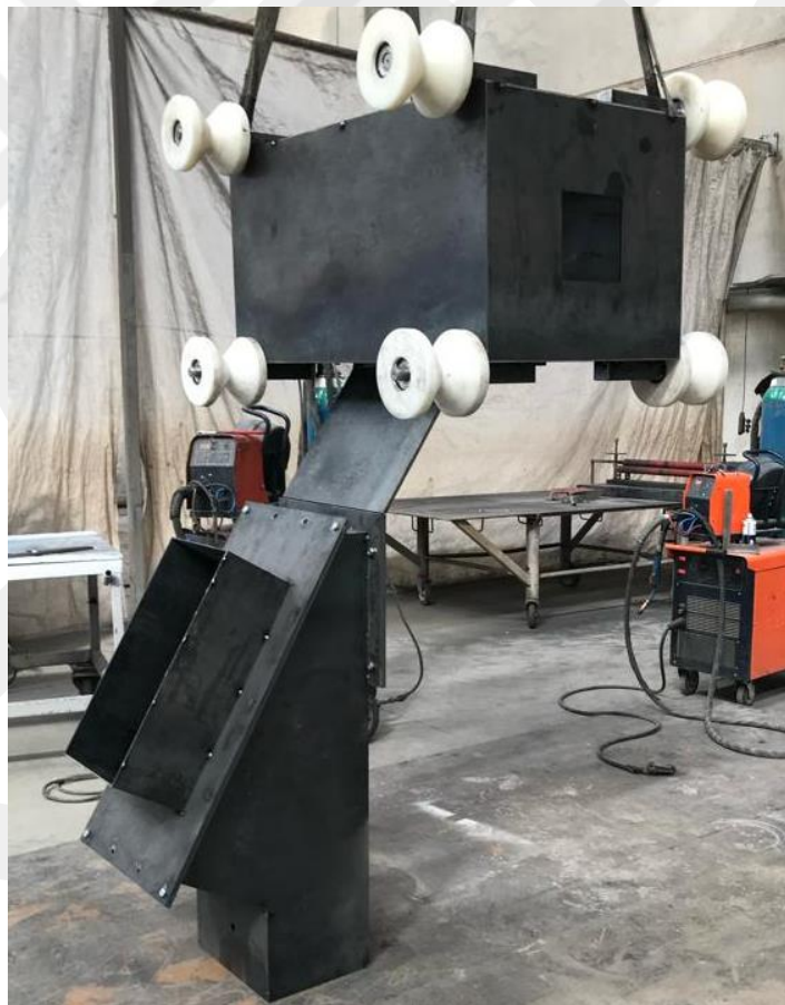
Figure 4.13: Assembling process of the sample receiver trolley, cutter, and chute.
