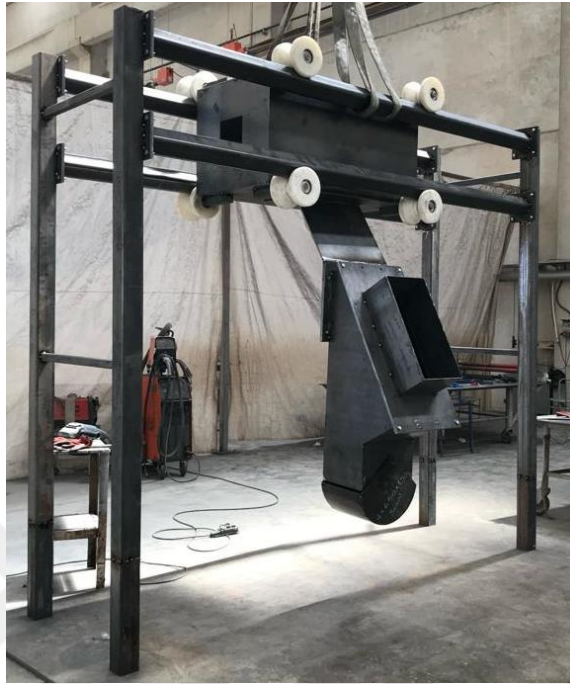
Figure 4.14: Assembling process of cutter, sample receiver trolley, chute, and steel structure.
