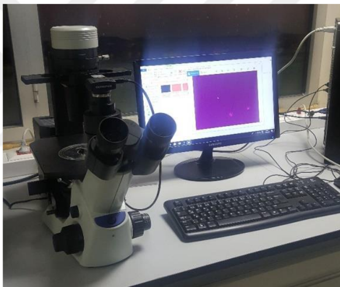
Figure 2.6. Inverted Microscope (Olympus CKX53 )
