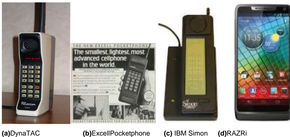
Figure 2.1: Milestones of the mobile phone evolution: (a) Motorola DynaTAC was the first mobile handheld phone commercially available, (b) an advertisement of the first mobile phone that would fit into a pocket, (c) the IBM Simon as first mobile phone that was referred to as a smartphone, and (d) the Motorola RAZRi as a representative of the current generation of smartphones.
