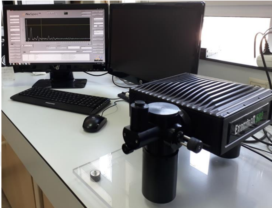
Figure (23) picture of the parts Raman spectrometer device
