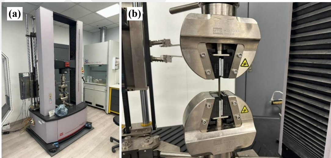
Figure 3.14 (a) MTS C45.305 tensile test machine (b) sample
