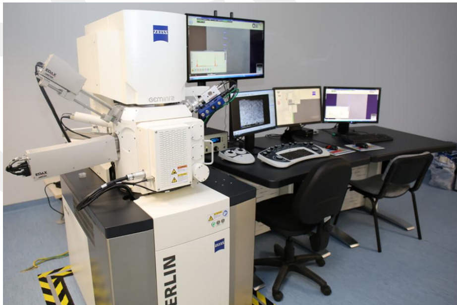
Figure 3.10 ZEISS MERLIN Scanning Electron Microscope (SEM) equipped with EDS and EBSD
