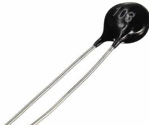
Figure 4.3 10k \Omega NTC thermistor
