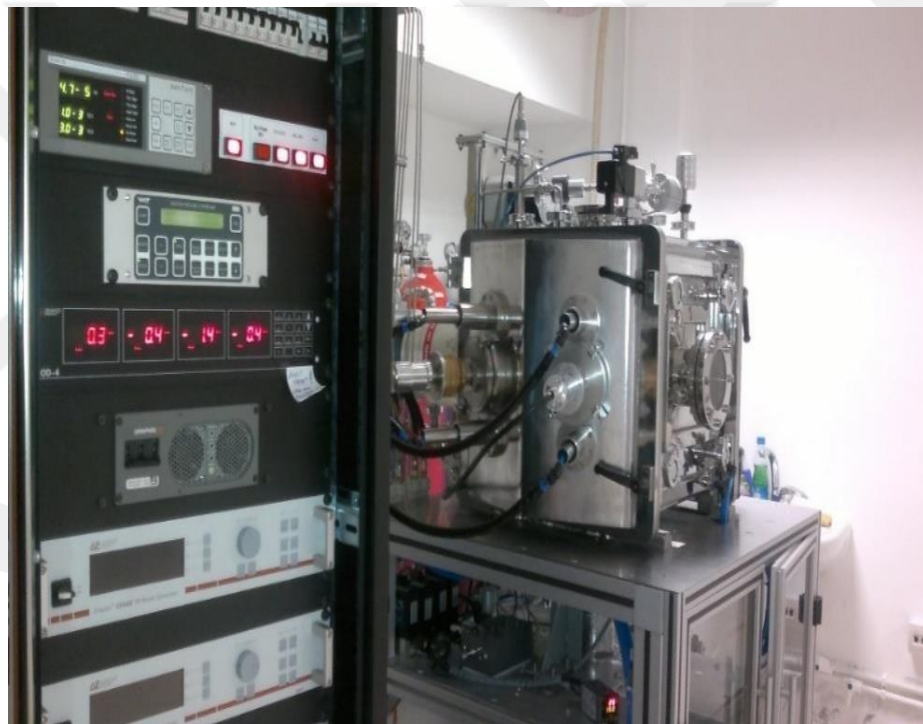
Figure 3.4 PVD coating system
