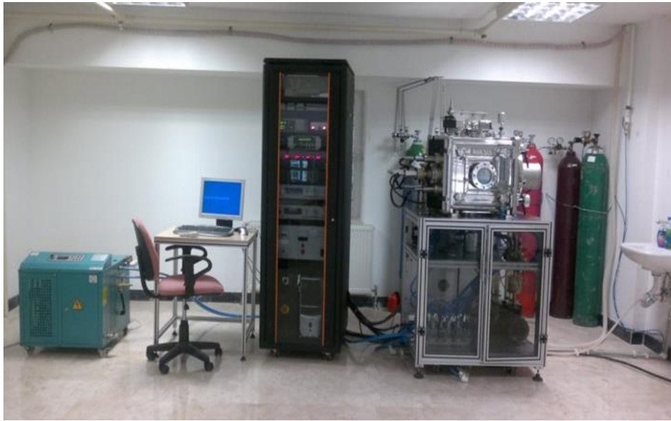
Figure 3.2 Parts of PVD magnetron sputtering system
