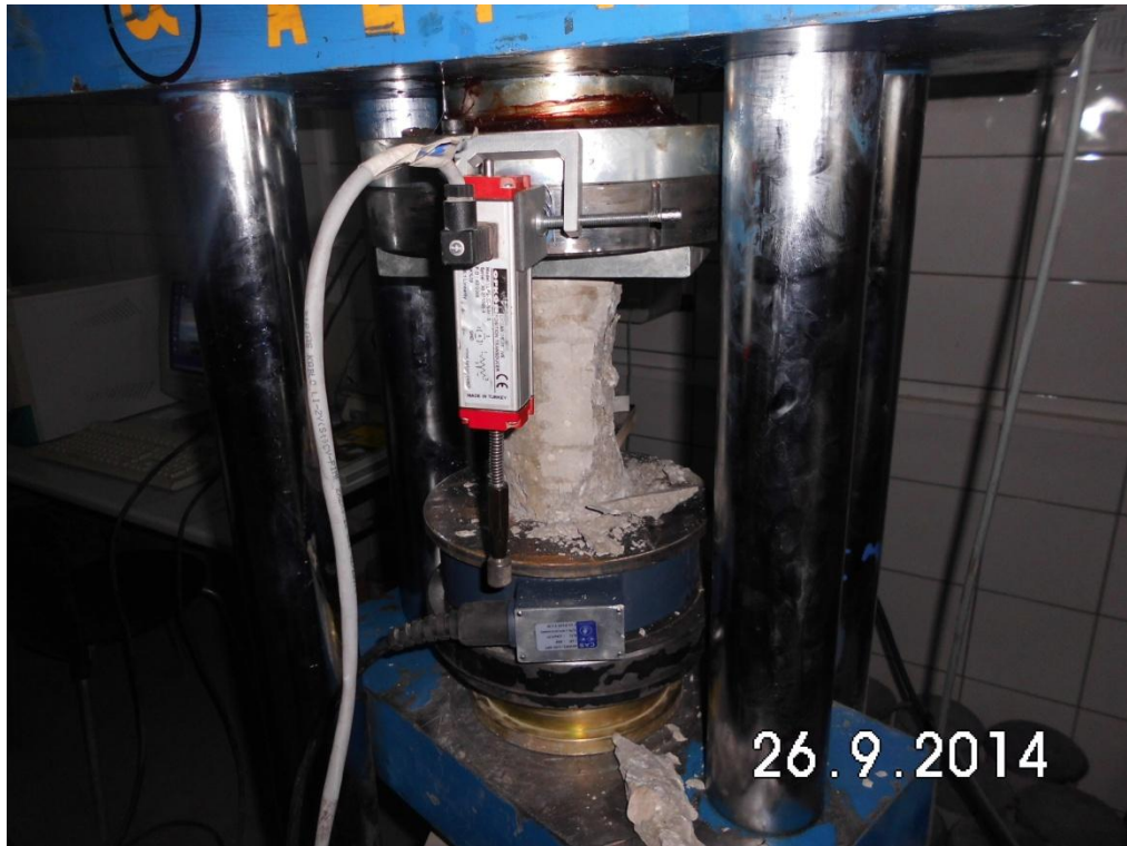
Figure 4-1 – Typical failure mode of CC cylinders under compression
