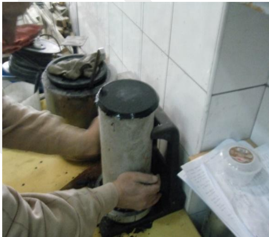
Figure 3-11 – Capping of 150×300 mm cylinders
