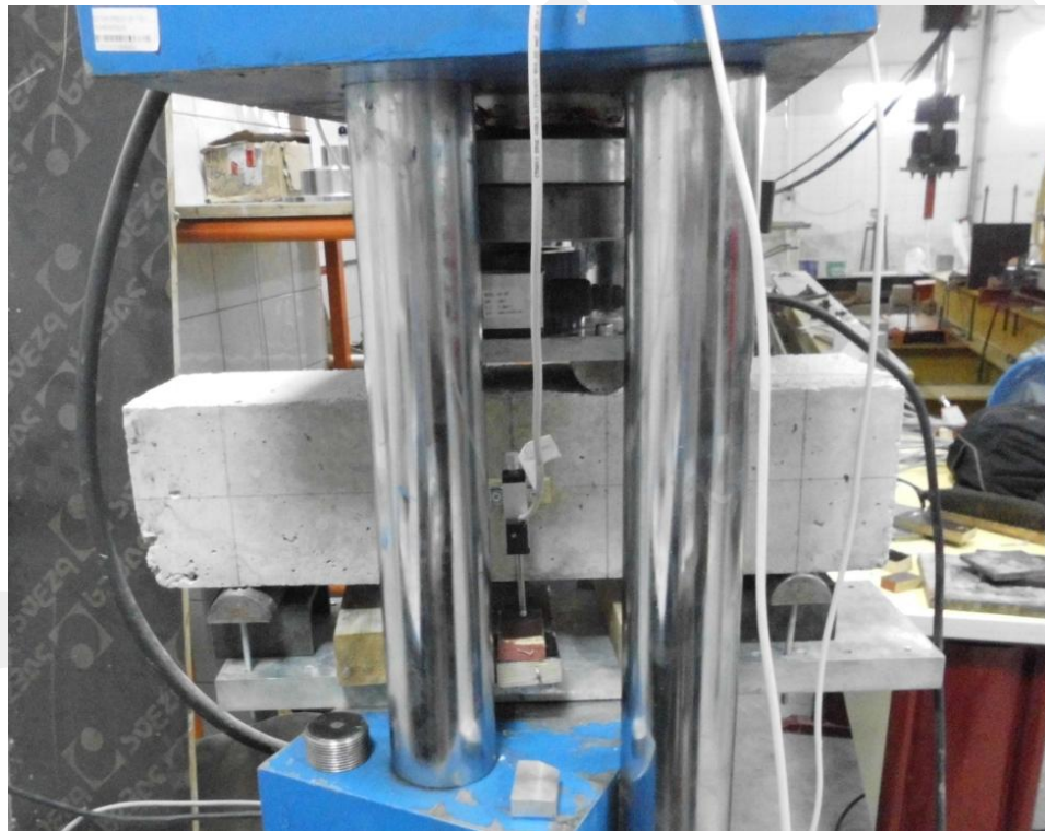
Figure 3-12 – Flexural beam tests (four-point bending)
