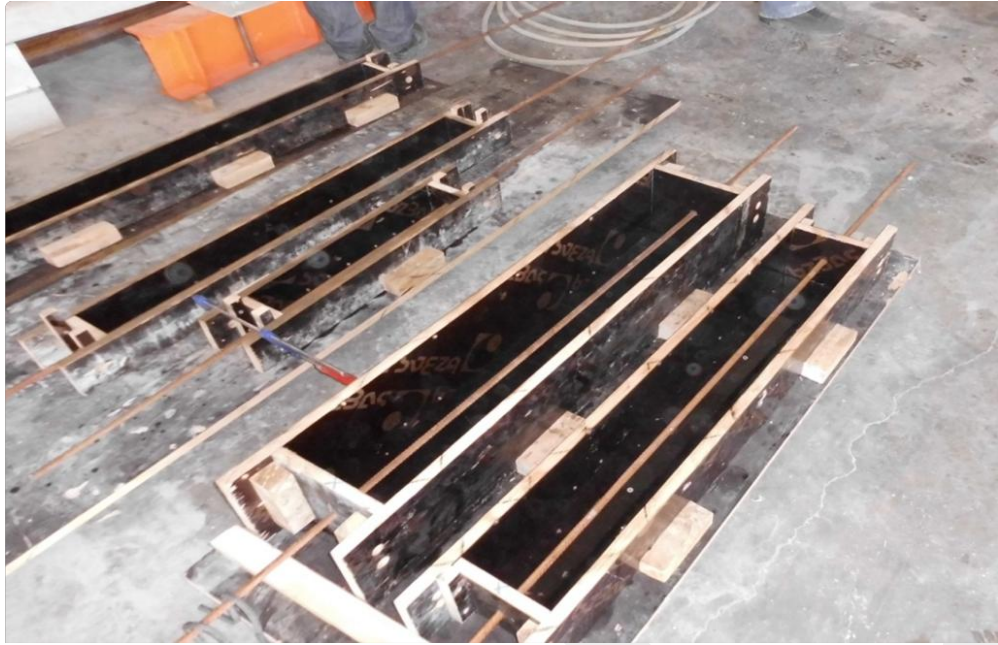
Figure 3-6 – Typical formworks for prismatic tension specimens with reinforcing bar
