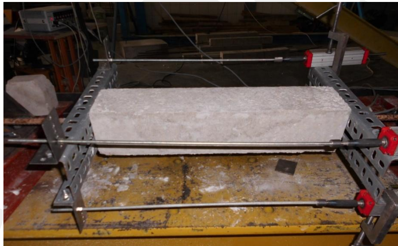
Figure 3-16 – Test set-up for prismatic tension specimens with bar
