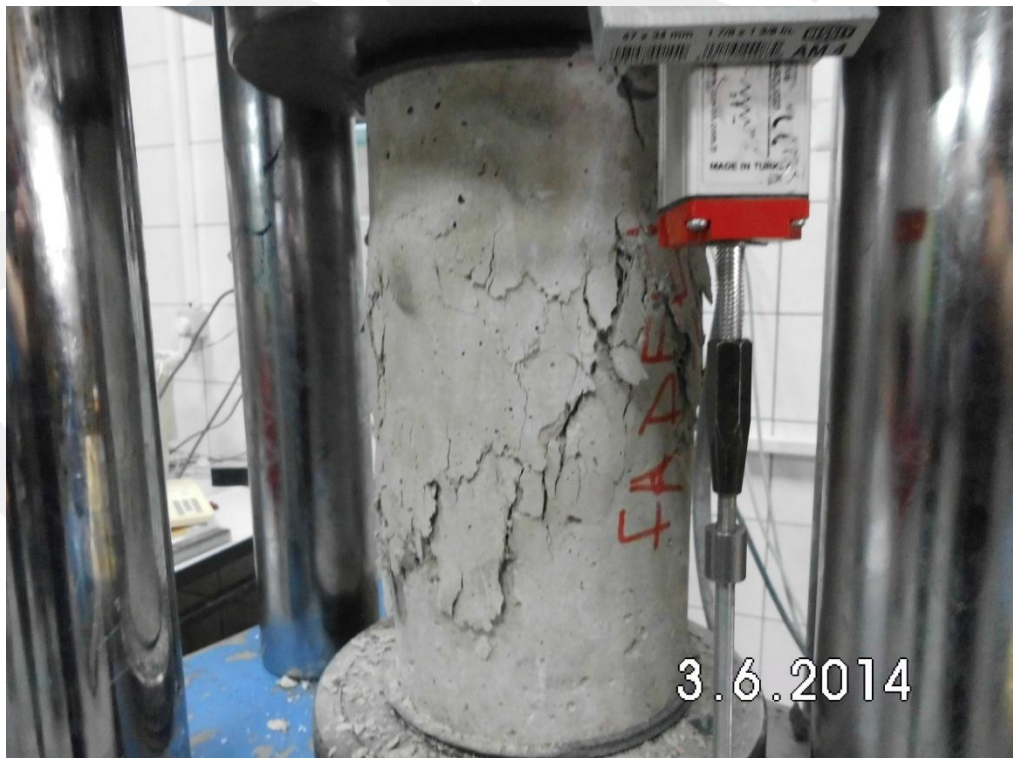
Figure 4-2 – Typical failure mode of SFRC cylinders under compression
