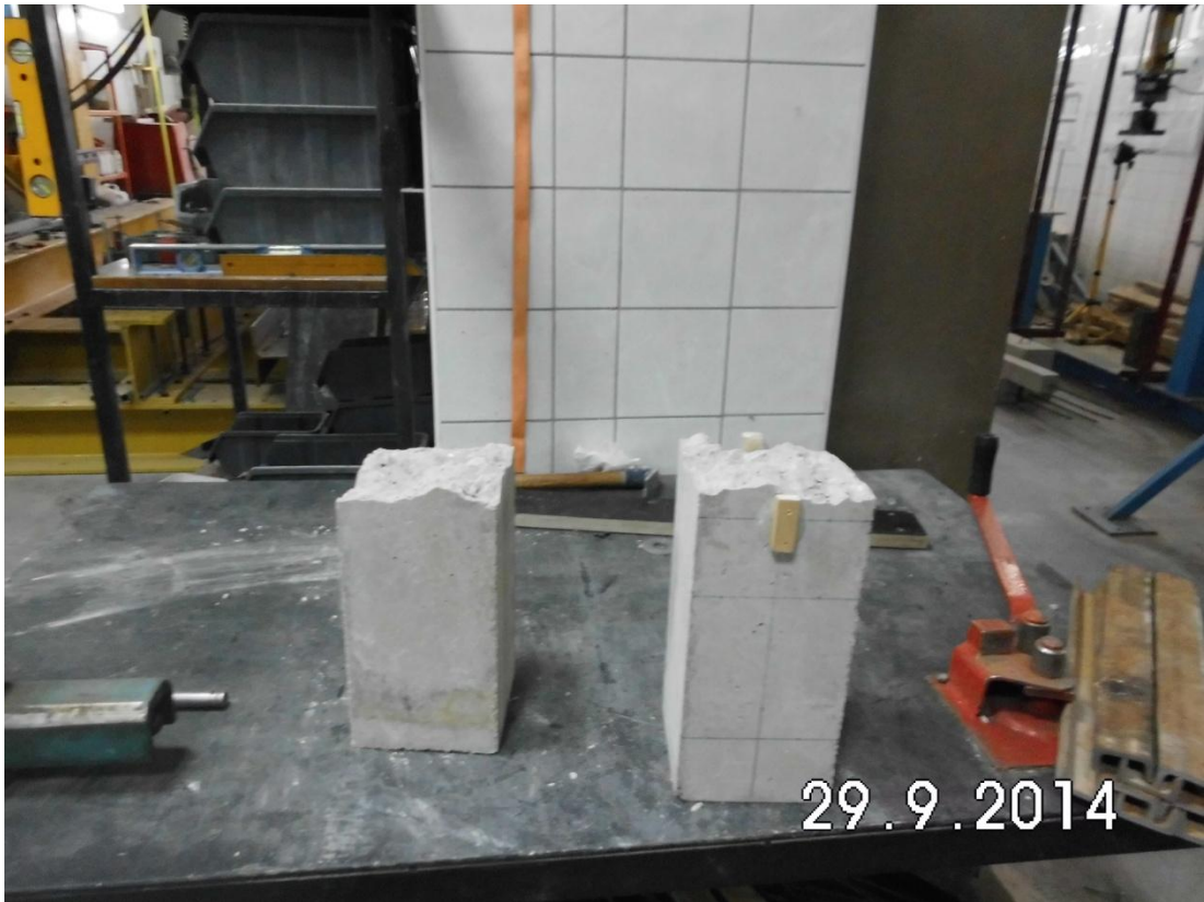
Figure 4-7 – Typical failure mode of CC flexural beams
