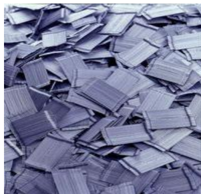
Figure 3-4 – Dramix ZP 305 steel fiber used in the research
