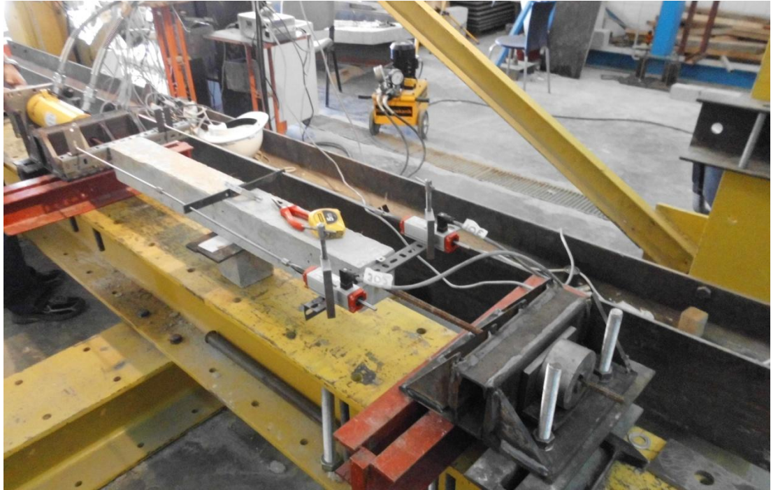
Figure 3-2 – General view of prismatic tension specimens with reinforcing bar
