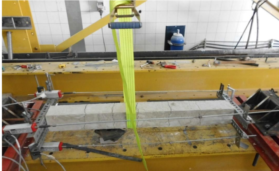
Figure 4-13 – Typical crack patterns for CC tension specimens (CC100×100×1000-01)
