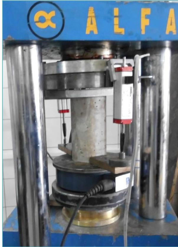
Figure 3-10 – Testing of cylinders
