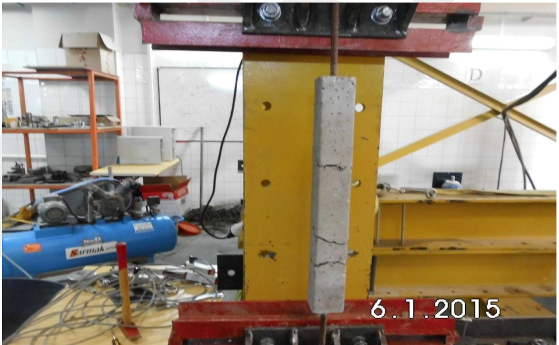
Figure 4-16 – Typical crack patterns for SFRC tension specimens (SFRC60×60×500-01)
