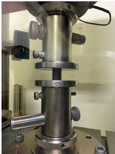
Figure 5. Uniaxial compression test setup
