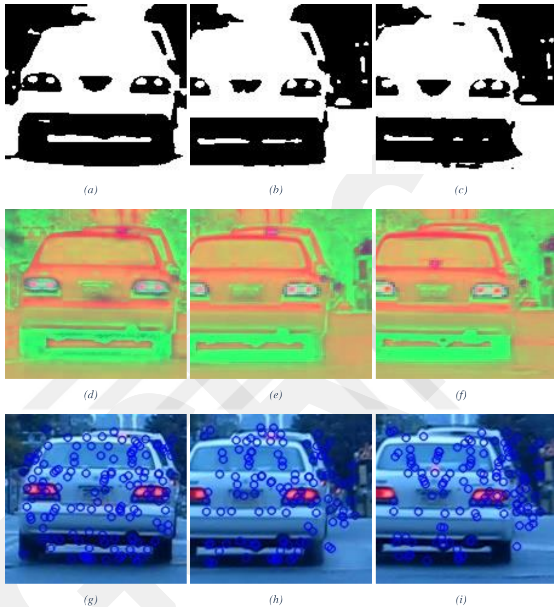
Figure 5-12 (a) Selected object from first frame in Template Matching. (b)(c) Detected object from 5. and 10. frame in Template Matching, respectively. (d) Selected object from first frame in Color-Based Histogram. (e)(f) Detected object from 5. and 10. frame in Color-Based Histogram, respectively. (g) Selected object from first frame in SURF. (h)(i) Detected object from 5. and 10. frame in SURF.
