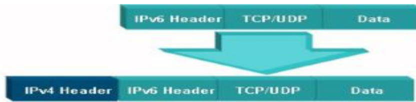
Figure 3.3: IPv6 over IPv4 Tunneling [28]
