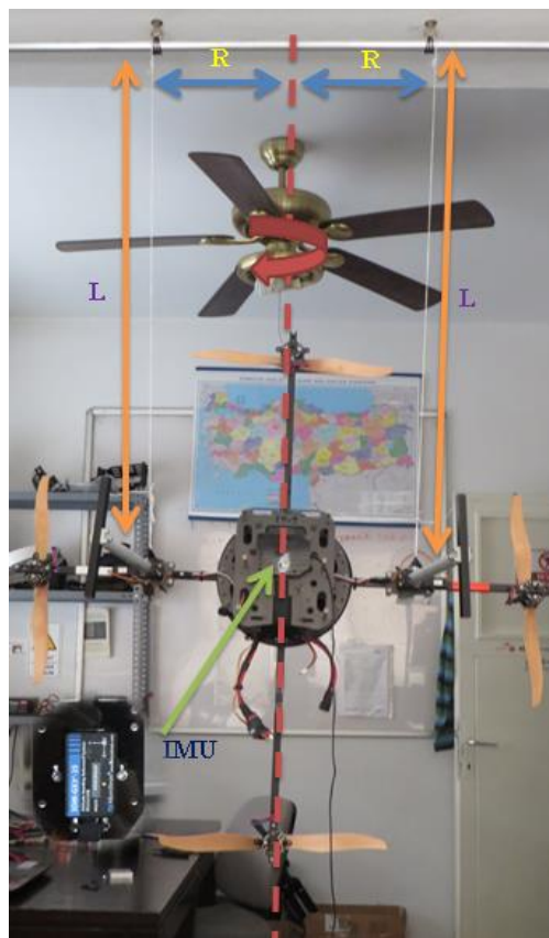
Figure 39: Inertia Test on Roll ( J_{xx} ) axis
