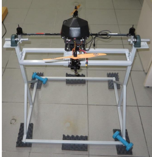
Figure 47: One Axis Test Bench
