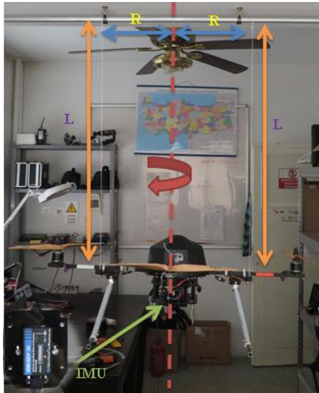
Figure 43: Inertia Test on Yaw ( J_{zz} ) axis
