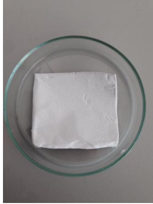
Figure 3.1. Macroscopic appearance of the electrospun PCL/chitosan core-shell scaffold.
