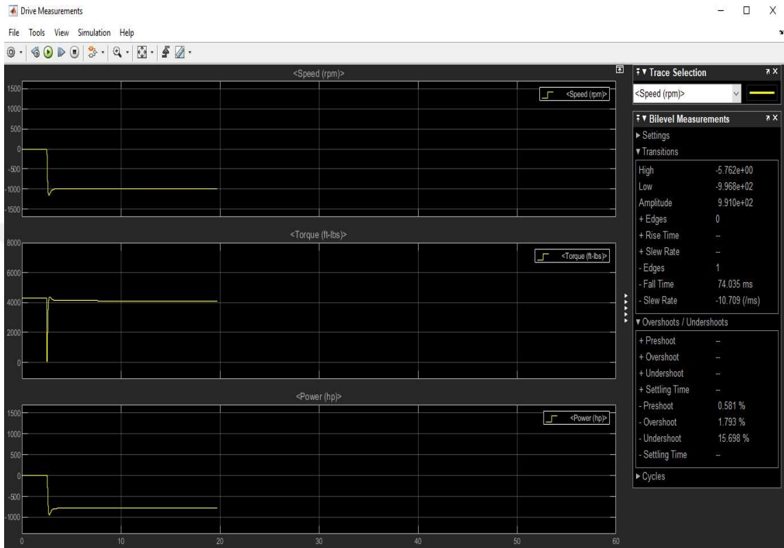
Figure 4.1 (j): Graph for speed, torque, and power at 1000 rpm
