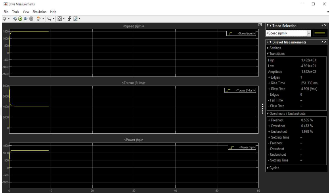
Figure 4.1 (b): Graph for speed, torque, and power at 1500 rpm
