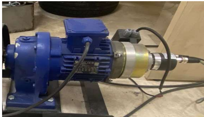
Figure 3.4.6 (c): AC motor type V2E-A-80-M-4-A
