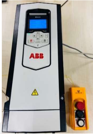
Figure 3.4.6 (g): ABB's type ACS880 motor drive
