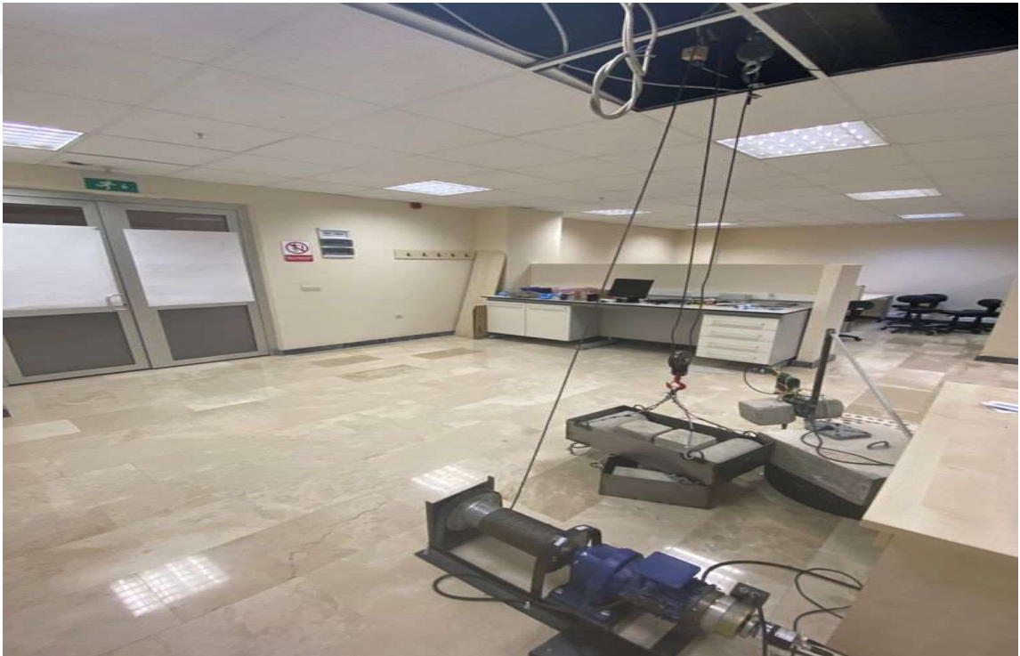
Figure 3.4.6 (a): Prototype model of drawworks control system
