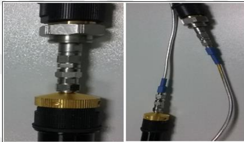
Figure 3.9. Measurement of the power loss due to used connectors and cables.
