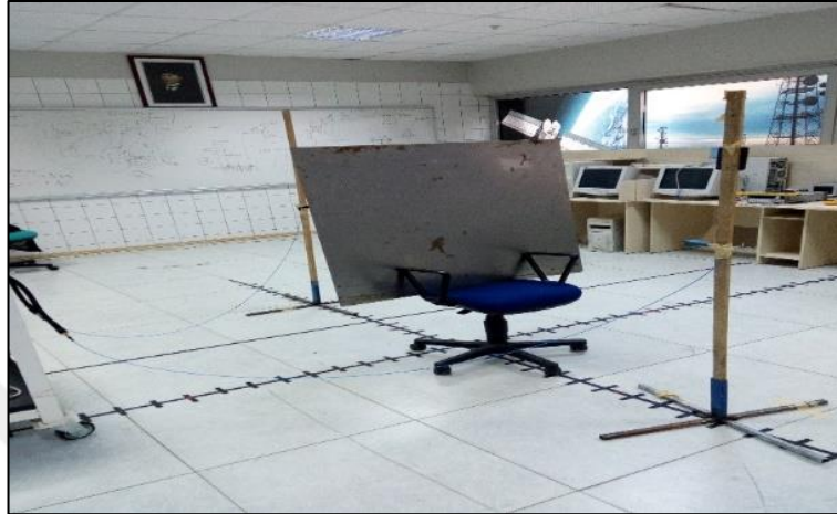
Figure 3.18. Full blockage LOS at center by plate of metal.
