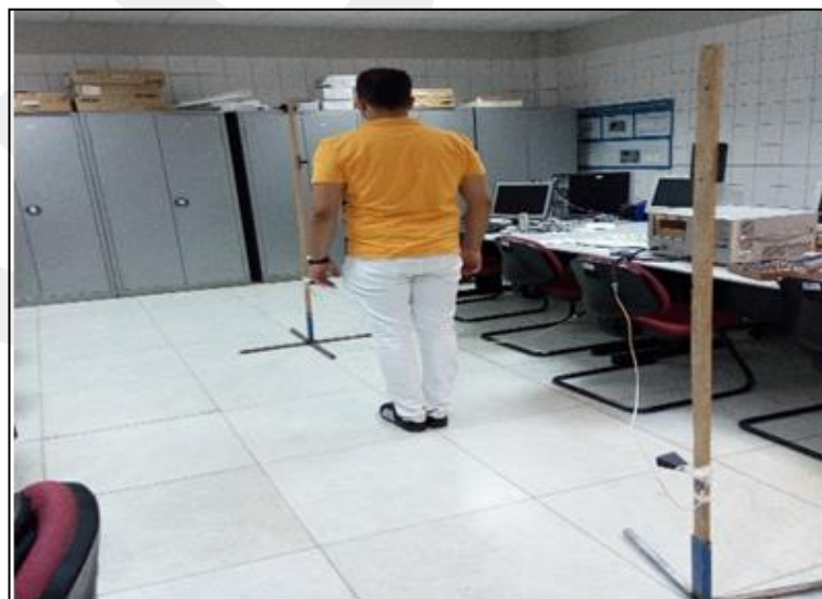
Figure 3.12. Radio link fully blocked by a person.
